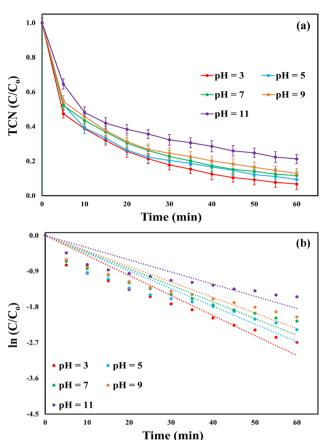
Fig. 6 Effect of pH on the catalytic efficiency of the MWLB (25)/PI system under the control conditions: (a) TCN removal percentages and (b)  $K_{\rm obs}$ .
