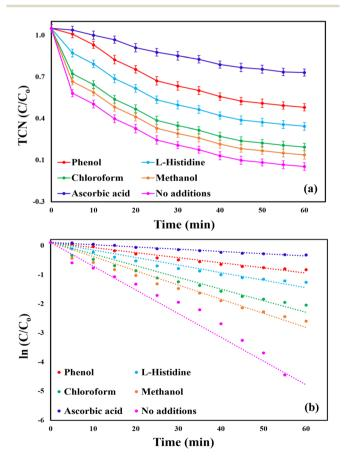
Fig. 11 Effect of various quenching agents (30 mM) on TCN degradation in the MWLB (25)/PI system under the optimum conditions: (a) removal ratios and (b) kinetic rate constants.
