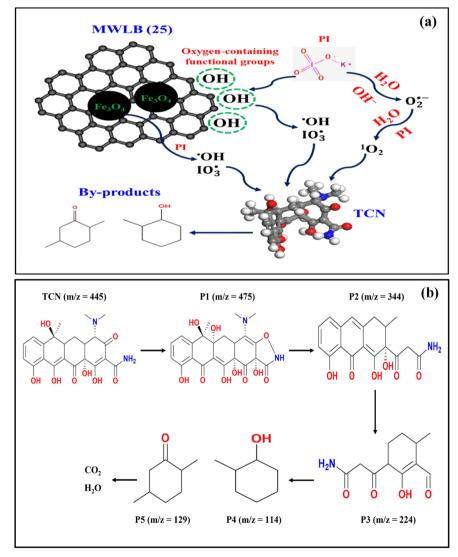
Fig. 12 (a) Degradation mechanism and (b) proposed TCN degradation pathways in the MWLB (25)/PI system.
