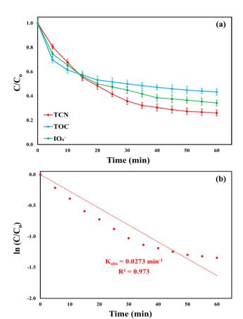
Fig. 14 Performance of the MWLB (25)/PI system in treating real pharmaceutical wastewater: (a) TCN degradation ratio, TOC mineralization efficiency, and  $\rm IO_4^-$  consumption; (b) apparent degradation rate constant of TCN. Conditions:  $\rm [TCN]_o=428.36~mg~L^{-1}$ ,  $\rm [TOC]_o=1372.298~mg~L^{-1}$ ,  $\rm pH=7$ ,  $\rm T=25$ ,  $\rm [catalyst]_o=0.83~g~L^{-1}$ ,  $\rm [PI]_o=2.05~mM$ .
