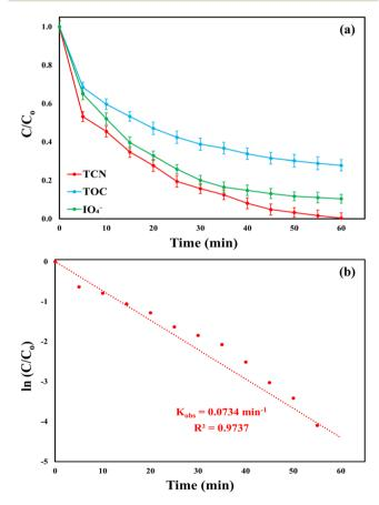
Fig. 8 (a) TCN degradation ratio, TOC mineralization efficiency, and  ${\rm IO_4}^-$  consumption rate; (b) kinetics of TCN degradation in the MWLB (25)/PI system under the optimum conditions:  ${\rm [TCN]_o}=16.52~{\rm mg~L^{-1}}$ ,  ${\rm [catalyst]_o}=0.83~{\rm g~L^{-1}}$ ,  ${\rm [PI]_o}=2.05~{\rm mM}$ , pH = 7,  $T=25~{\rm ^{\circ}C}$ , and  ${\rm [TOC]_o}=8.83~{\rm mg~L^{-1}}$ .
