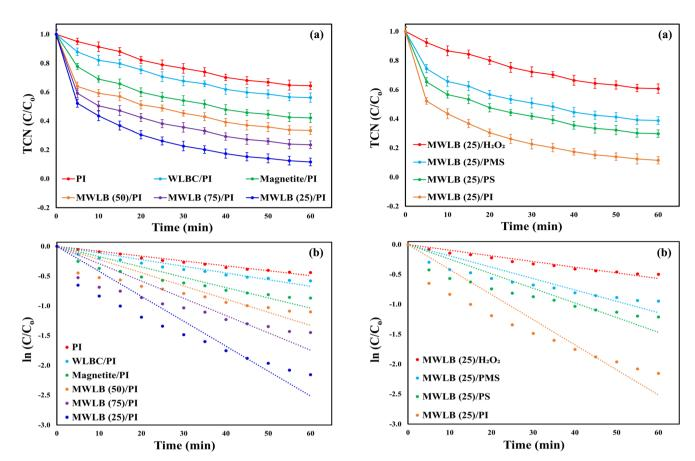
Fig. 4 Control experiments: (a) TCN removal efficiency and (b) kinetic analysis. Conditions:  $[TCN]_o = 20 \text{ mg L}^{-1}$ ,  $[catalyst]_o = 0.75 \text{ g L}^{-1}$ ,  $[PI]_o = 1.5 \text{ mM}$ , pH = 7, and  $T = 25 ^{\circ}C$ .
