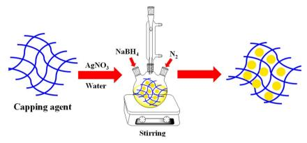
Fig. 4 Synthesis of silver nanoparticles in microgels by in situ reduction method.
