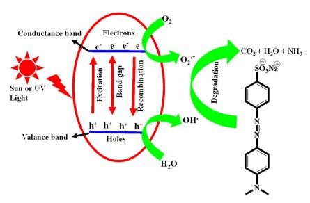
Fig. 8 Photocatalytic degradation mechanism of methyl orange.
