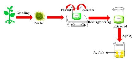
Fig. 2 Synthesis of silver nanoparticles with the help of plant extract.
