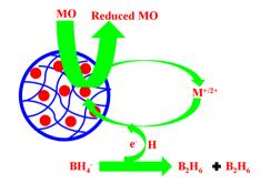
Fig. 7 Catalytic reduction mechanism of methyl orange in the presence of NaBH<sub>4</sub> and metallic nanocatalyst in capping agent.
