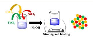
Fig. 5 Fe/Co/Ni tri-metal nanoparticles synthesis. 133
