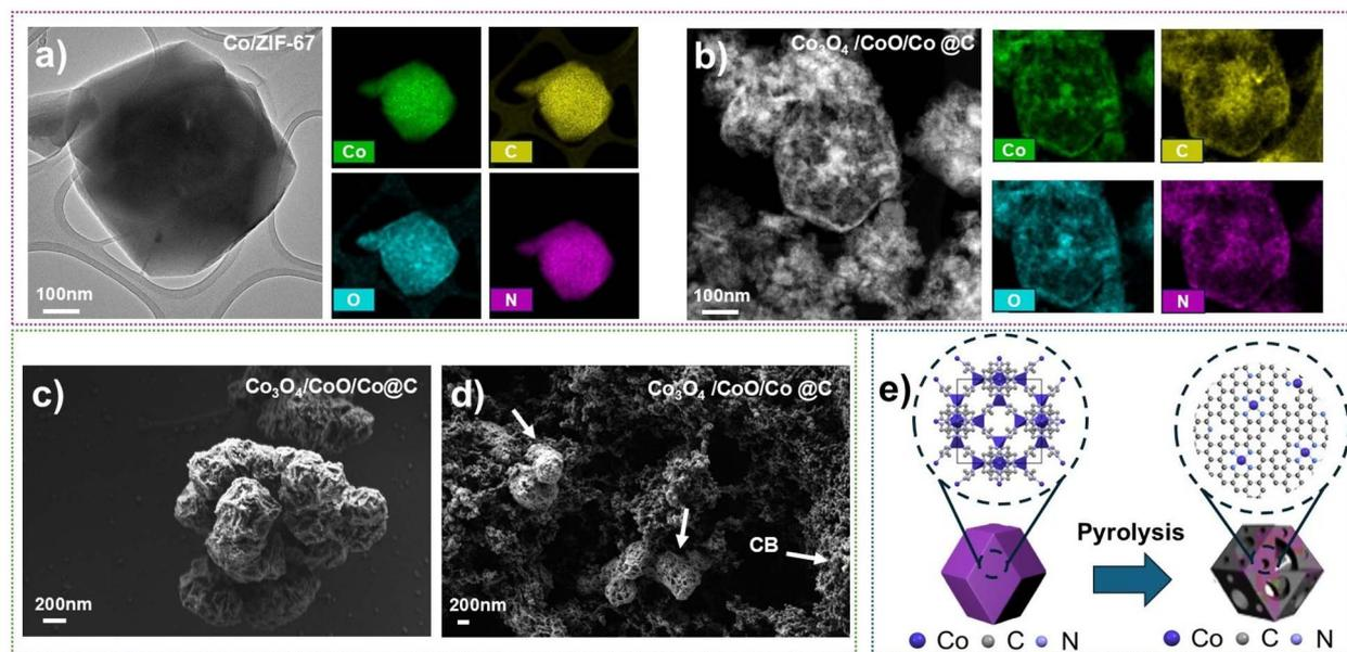
Fig. 4 (a) Elemental mapping of Co/ZIF-67 before pyrolysis, (b) SEM micrographs of  $\text{Co}_3\text{O}_4/\text{CoO}/\text{Co}@C$  HNCs after pyrolysis at  $500\text{ }^\circ\text{C}$  under  $\text{N}_2$ , (c) SEM micrograph of pyrolyzed sample before, and (d) after carbon black addition, (e) schematic illustration of the final Co/ZIF-67 and  $\text{Co}_3\text{O}_4/\text{CoO}/\text{Co}@C$  catalyst structure after pyrolysis.
