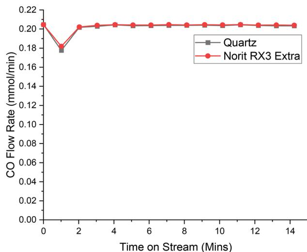
Fig. 4 The response of directing a flow of 5 ml per min CO in 54 ml per min  $\text{N}_2$  over a reactor containing ground quartz (black) and the Norit RX3 Extra formulation of activated carbon (red), at 323 K. 0.4410 g of quartz was used, ground to between 250 and 500  $\mu\text{m}$ . 0.1250 g of Norit RX3 Extra, ground to between 250 and 500  $\mu\text{m}$ . The associated spectra are presented in Fig. S6 and S7.†
