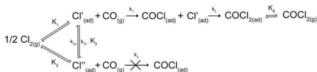
**Scheme 1** A reaction model for phosgene synthesis from carbon monoxide and chlorine over activated carbon. Reproduced with permission from *ref.* 33.
