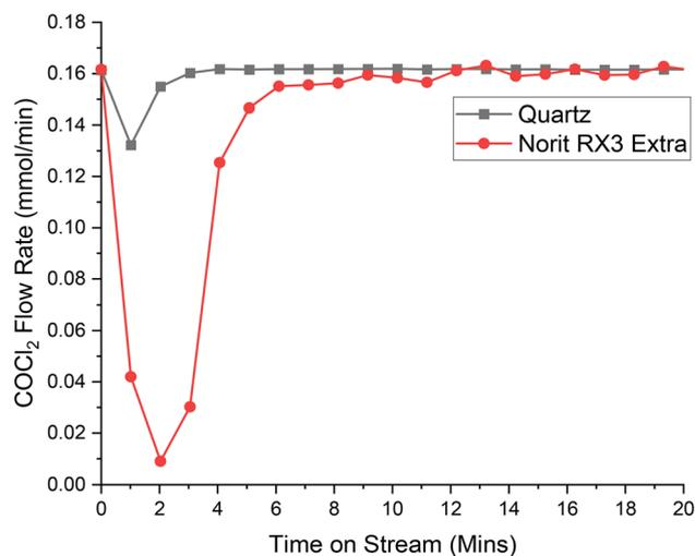
Fig. 6 The response of directing a flow of 40 ml  $\text{min}^{-1}$  of 10%  $\text{COCl}_2$  in He (4 ml per min  $\text{COCl}_2$ ) and 19 ml per min  $\text{N}_2$  over a reactor containing ground quartz (black) and the Norit RX3 Extra formulation of activated carbon (red), at 323 K. 0.4410 g of quartz was used, ground to between 250 and 500  $\mu\text{m}$ . 0.1250 g of Norit RX3 Extra, ground to between 250 and 500  $\mu\text{m}$ . The associated spectra are presented in Fig. S12 and S13.†
