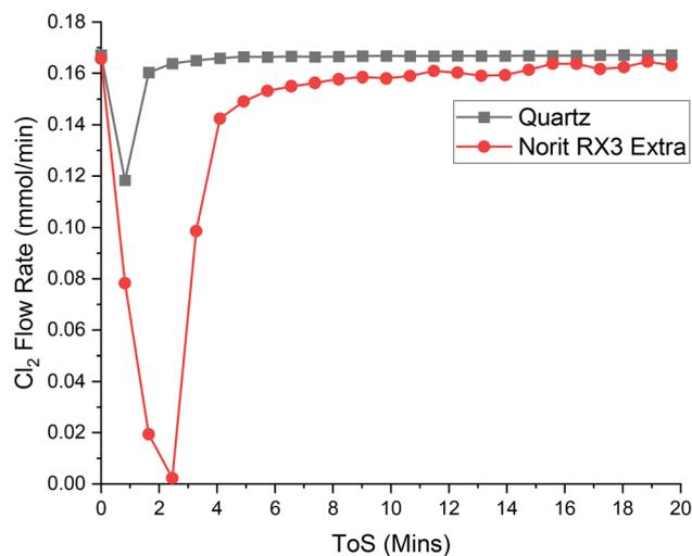
Fig. 5 The response of directing a flow of 4 ml per min  $\text{Cl}_2$  in 55 ml per min  $\text{N}_2$  over a reactor containing ground quartz (black) and the Norit RX3 Extra formulation of activated carbon (red), at 323 K. 0.4410 g of quartz was used, ground to between 250 and 500  $\mu\text{m}$ . 0.1250 g of Norit RX3 Extra, ground to between 250 and 500  $\mu\text{m}$ . The associated spectra are presented in Fig. S8 and S9.†
