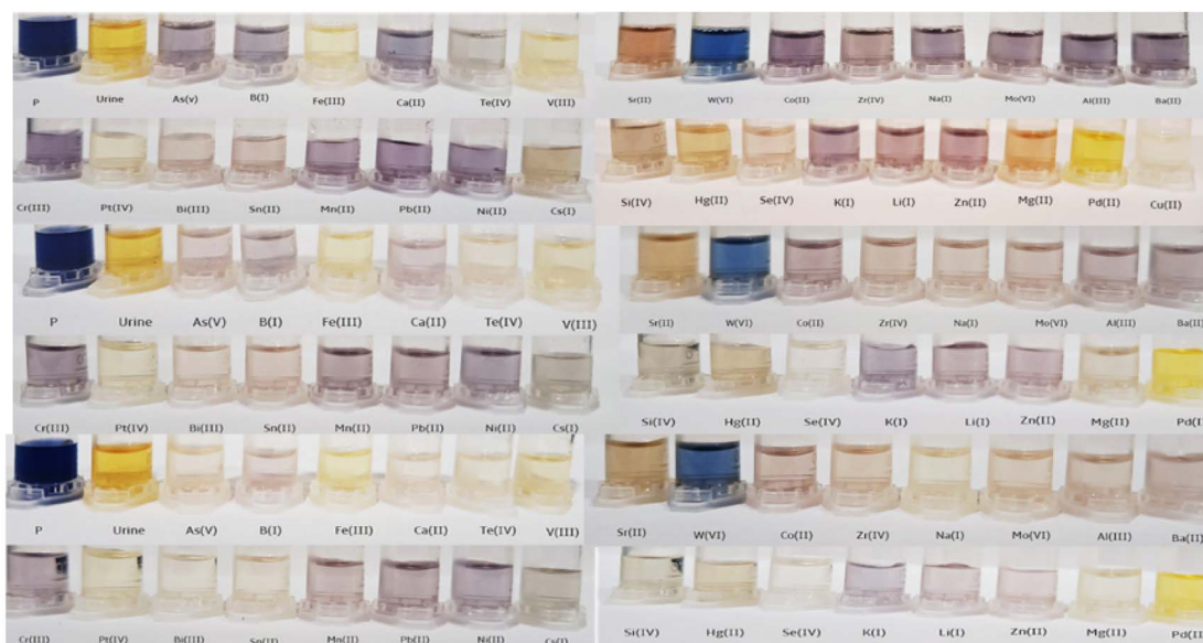
Fig. 9 Colorimetric assay of T-AgNPrs-DES as a sensing probe to identify different ions in human urine samples by the Spike method at three distinct incubation reaction times (0, 30, and 60 minutes).
