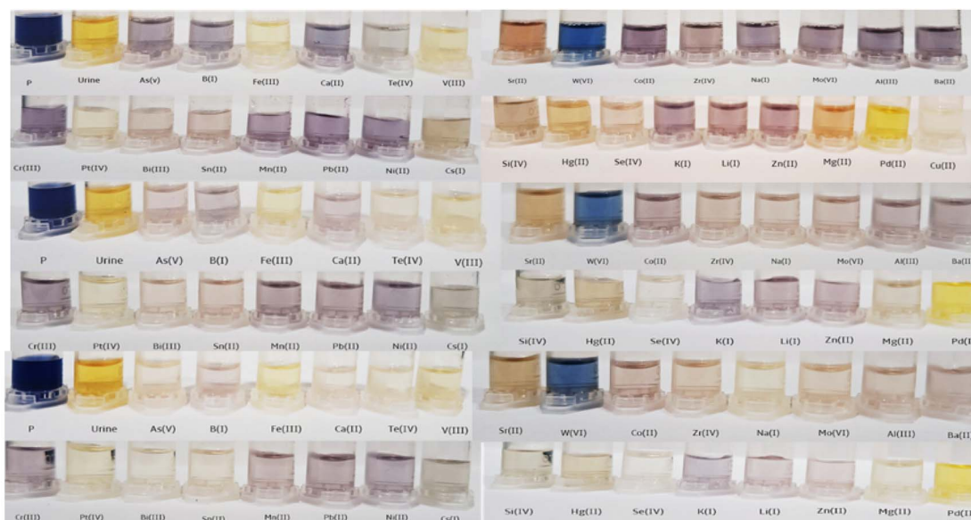
Fig. 9 Colorimetric assay of T-AgNPrs-DES as a sensing probe to identify different ions in human urine samples by the Spike method at three distinct incubation reaction times (0, 30, and 60 minutes).
