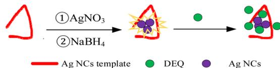
Scheme 1 Schematic diagram of the DEQ detection process.
