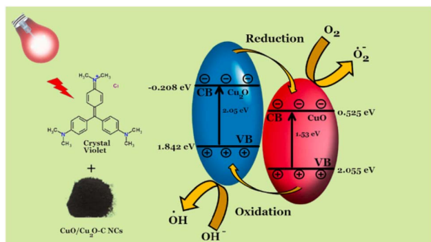
Fig. 10 Mechanism of degradation between CV and copper nanoparticles.
