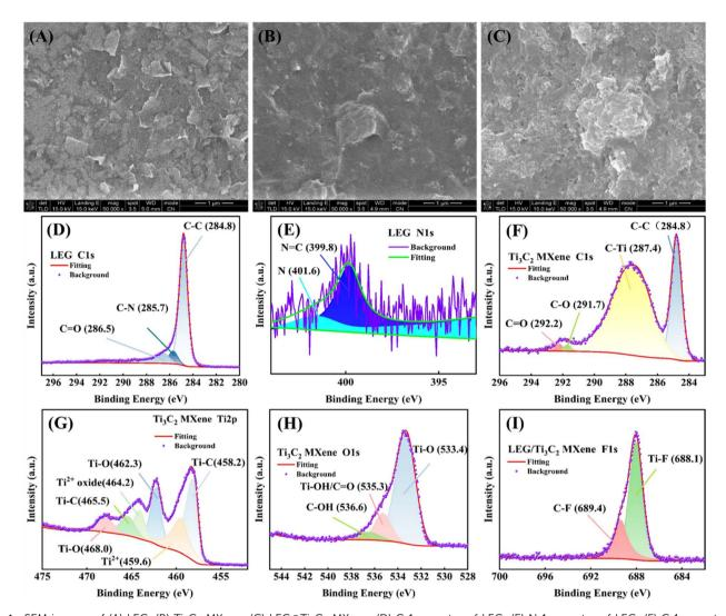
Fig. 1 SEM images of (A) LEG, (B)  $Ti_3C_2$  MXene, (C) LEG@ $Ti_3C_2$  MXene. (D) C 1s spectra of LEG; (E) N 1s spectra of LEG; (F) C 1s spectra of LEG@ $Ti_3C_2$  MXene; (G) Ti 2p spectra of  $Ti_3C_2$  MXene; (H) O 1s spectra of  $Ti_3C_2$  MXene; (I) F 1s spectra of LEG@ $Ti_3C_2$  MXene  $Ti_3C_2$  MXene.
