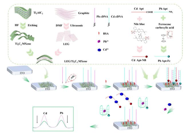
Scheme 1 Schematic diagram of the duplex electrochemical aptasensor for simultaneous detection of Cd<sup>2+</sup> and Pb<sup>2+</sup> ions.
