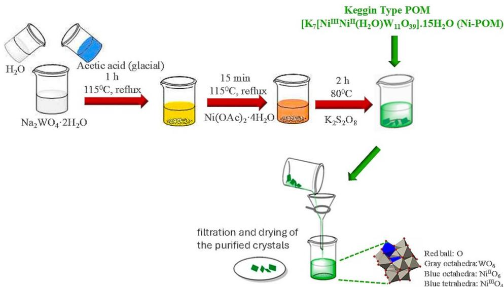
Scheme 1 Illustration of the synthesis procedure of Ni-POM.
