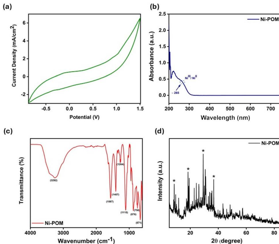
Fig. 1 (a) CV of Ni-POM ( $10^{-3}$  M) in acetonitrile on graphite electrode using  $\text{Bu}_4\text{NBF}_4$  ( $10^{-1}$  M) as the support electrolyte. (b) UV-spectrum of Ni-POM in water. (c) FT-IR spectra of Ni-POM. (d) XRD patterns of Ni-POM.
