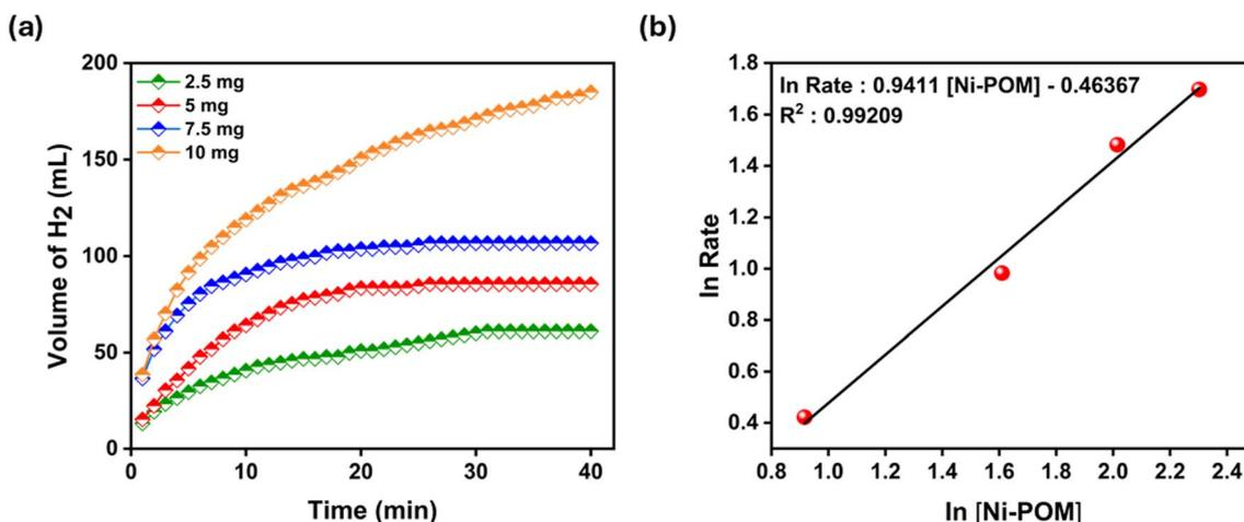
Fig. 6 (a)  $\text{H}_2$  production volume versus time graph in the presence of different amounts of catalysts [ $\text{NaBH}_4$  concentration 300 mM, 25 °C] and (b) logarithmic ratio of hydrogen release *versus* logarithmic concentration of Ni-POM for  $\text{NaBH}_4$  hydrolysis.
