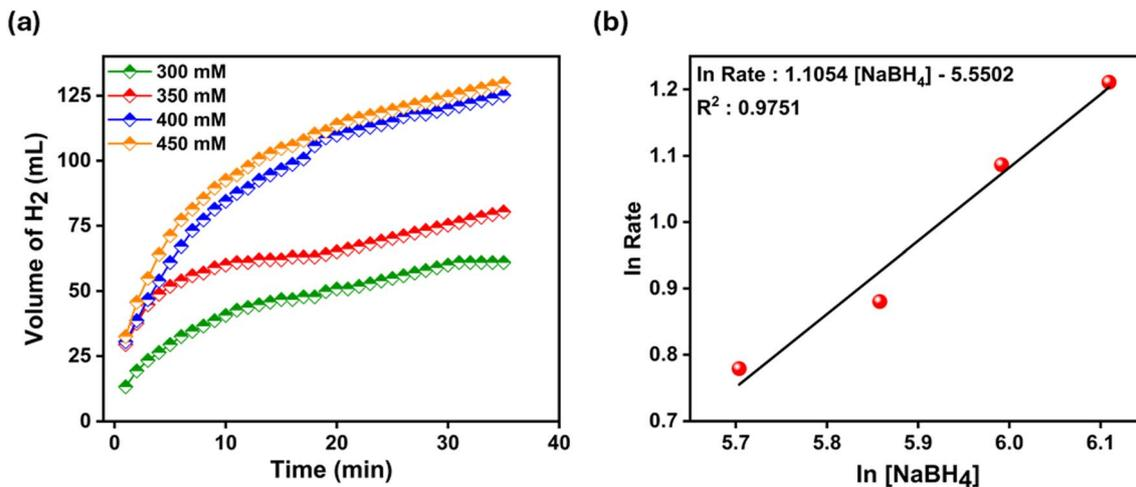
Fig. 7 (a) H<sub>2</sub> production volume versus time graph at different NaBH<sub>4</sub> concentrations [Ni-POM 2.5 mg, 25 °C] and (b) logarithmic ratio of hydrogen release versus logarithmic concentration of NaBH<sub>4</sub> for NaBH<sub>4</sub> hydrolysis.
