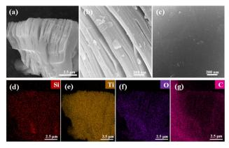
Fig. 2 SEM images of MXene@SiO $_2$  (a-c), EDS of images of Si, Ti, O, C elements for MXene@SiO $_2$  composites: (d-q).
