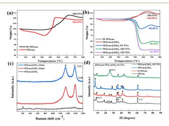
Fig. 4 TG of MXene, H-MXene, MXene@SiO $_2$  and MXene@SiO $_2$ -CNTs composites (a and b), Raman of MXene@SiO $_2$  and MXene@SiO $_2$ -CNTs composites (c), XRD of MXene, H-MXene, MXene@SiO $_2$  and MXene@SiO $_2$ -15CNTs (d).
