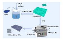
Fig. 1 The schematic diagram of the synthesis process of MXene@SiO $_2$ -CNTs composites.
