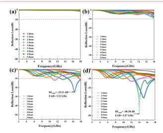
Fig. 6 Reflection loss plots of (a) pure MXene and (b-d) MXene@SiO<sub>2</sub>-CNTs with reaction time of respectively 5, 10, 15 min.
