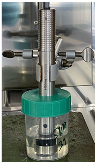
Fig. 1 Experimental set-up for conducting in-line UV-vis measurements in real time.
