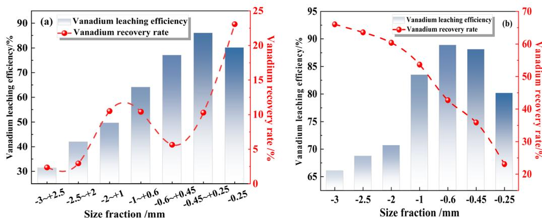
Fig. 5 The vanadium leaching efficiency for different particle sizes with 30 wt% H<sub>2</sub>SO<sub>4</sub>, 5 wt% CaF<sub>2</sub>, a leaching temperature of 98 °C and a leaching time of 12 h (a) narrow particle size and (b) wide particle size).
