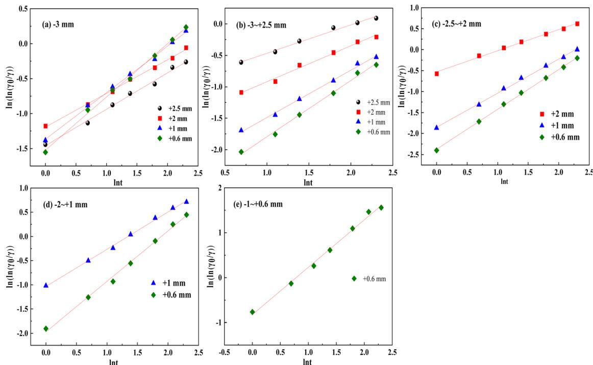
Fig. 9 Fitting curve of the grinding kinetics of vanadium-bearing shale (feed particle size: (a):  $-3$  to  $+0.6$  mm; (b):  $-3$  to  $+2.5$  mm; (c):  $-2.5$  to  $+2$  mm; (d):  $-2$  to  $+1$  mm; (e):  $-1$  to  $+0.6$  mm).
