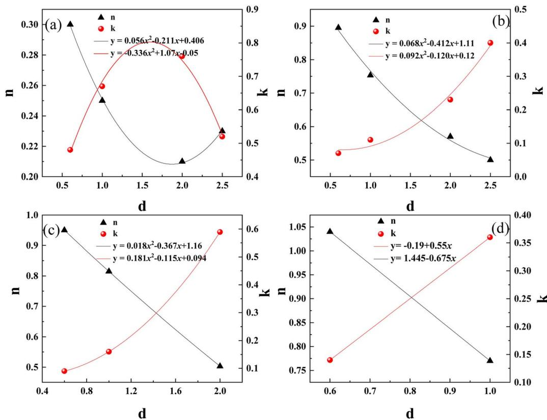
Fig. 10 The curve of the relationship between the grinding kinetics parameters  $n$  and  $k$  and the particle size  $d$  (feed particle size: (a):  $-3$  mm; (b):  $-3$  to  $+2.5$  mm; (c):  $-2.5$  to  $+2$  mm; (d):  $-2$  to  $+1$  mm).
