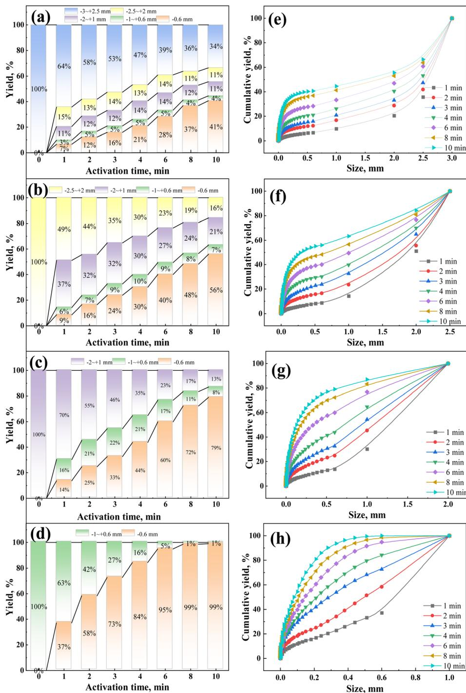
Fig. 8 The yields and cumulative yields of different particle size distribution under different activation times (graded particle size: (a and e):  $-3$  to  $+2.5$  mm; (b and f):  $-2.5$  to  $+2$  mm; (c and g):  $-2$  to  $+1$  mm; (d and h):  $-1$  to  $+0.6$  mm).
