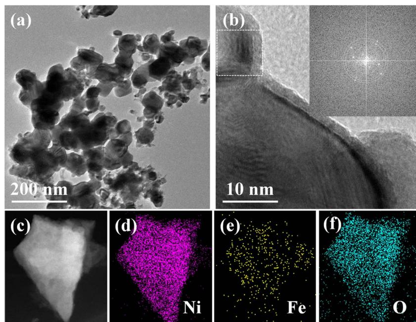
Fig. 3 TEM (a), HRTEM (b), HAADF image (c) and corresponding elemental mapping (d–f) of NiFe PBA-Ar/O<sub>2</sub>.
