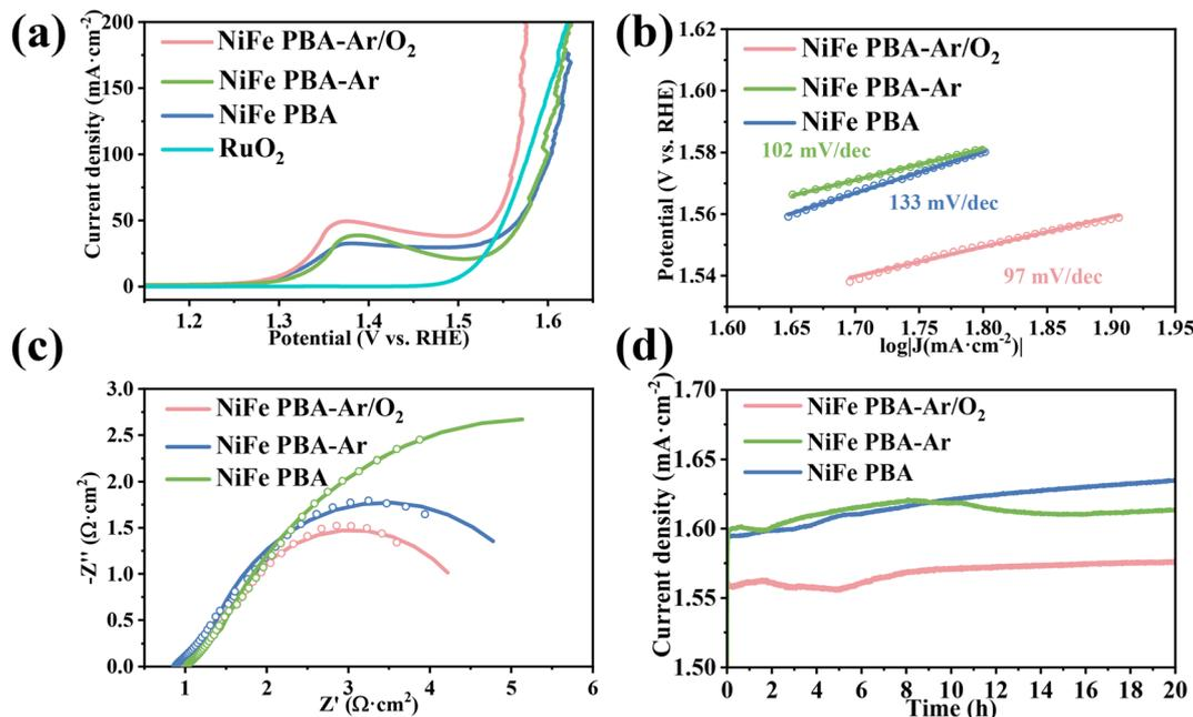
Fig. 5 LSV curves of NiFe PBA, NiFe PBA-Ar and NiFe PBA-Ar/O<sub>2</sub> catalysts in 1 M KOH solution (a); Tafel slope (b); EIS spectrum (c) and stability test curve (d).
