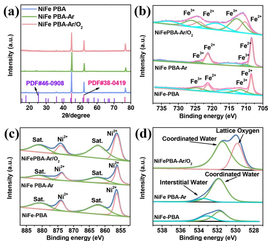
Fig. 4 XRD patterns of NiFe PBA, NiFe PBA-Ar and NiFe PBA-Ar/O<sub>2</sub> (a); fine spectra of Fe 2p (b), Ni 2p (c), and O 1s (d) XPS in NiFe PBA, NiFe PBA-Ar, and NiFe PBA-Ar/O<sub>2</sub> catalysts.
