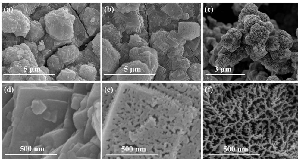
Fig. 2 SEM photographs of catalysts NiFe PBA (a and d), NiFe PBA-Ar (b and e) and NiFe PBA-Ar/O<sub>2</sub> (c and f).
