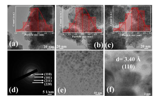
Fig. 2 HRTEM images of (a) Ag-00 ( $SnO_2$ ), (b) Ag-03 ( $SnO_2$ ), and (c) Ag-06 ( $SnO_2$ ) QDs, (d-f) SAED pattern, distinguish QDs and interplanar spacing of Ag-06 ( $SnO_2$ ) QDs.
