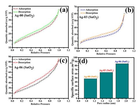
Fig. 7 (a-c) N<sub>2</sub> adsorption-desorption isotherms of all the samples and (d) histogram of the specific surface against pore radius.
