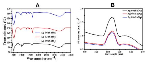
Fig. 5 (A) Stacked FTIR spectra (B) photoluminescence spectra of SnO<sub>2</sub> QDs and Ag-doped SnO<sub>2</sub> QDs.
