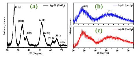
Fig. 1 P-XRD patterns of (a) Ag-00 (SnO<sub>2</sub>), (b) Ag-03 (SnO<sub>2</sub>), and (c) Ag-06 (SnO<sub>2</sub>) QDs.
