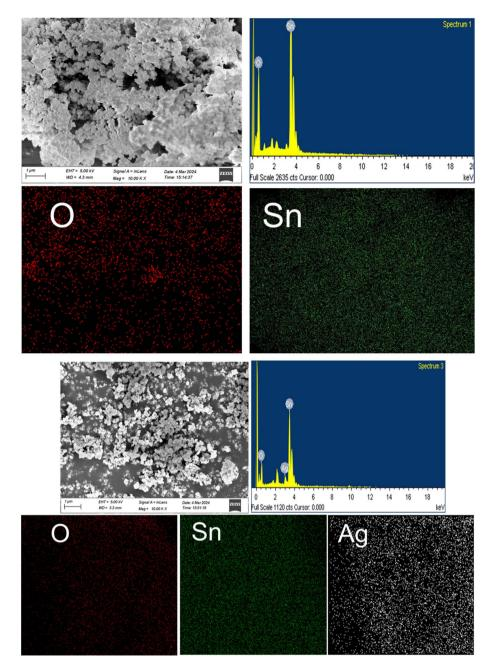
Fig. 6 (a) Pure SnO<sub>2</sub> QDs SEM image. (b) Ag-doped SnO<sub>2</sub> QDs [Ag-06(SnO<sub>2</sub>)] SEM image.
