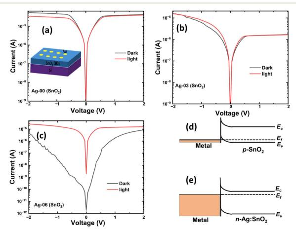
Fig. 10 (a–c) Current–voltage characteristics of  $SnO_2$  devices under dark and light conditions. Inset of 10 (a) depicts the schematic device configuration of  $Si/SnO_2$  (d) and (e) energy band diagram of  $SnO_2$  and Ag modified  $SnO_2$  devices.
