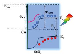
Fig. 11 Schematic energy band diagram of SnO<sub>2</sub> under the source.
