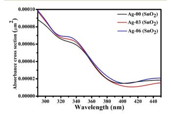
Fig. 3 Absorption cross-section of  $SnO_2$  QDs and Ag-doped  $SnO_2$  QDs.
