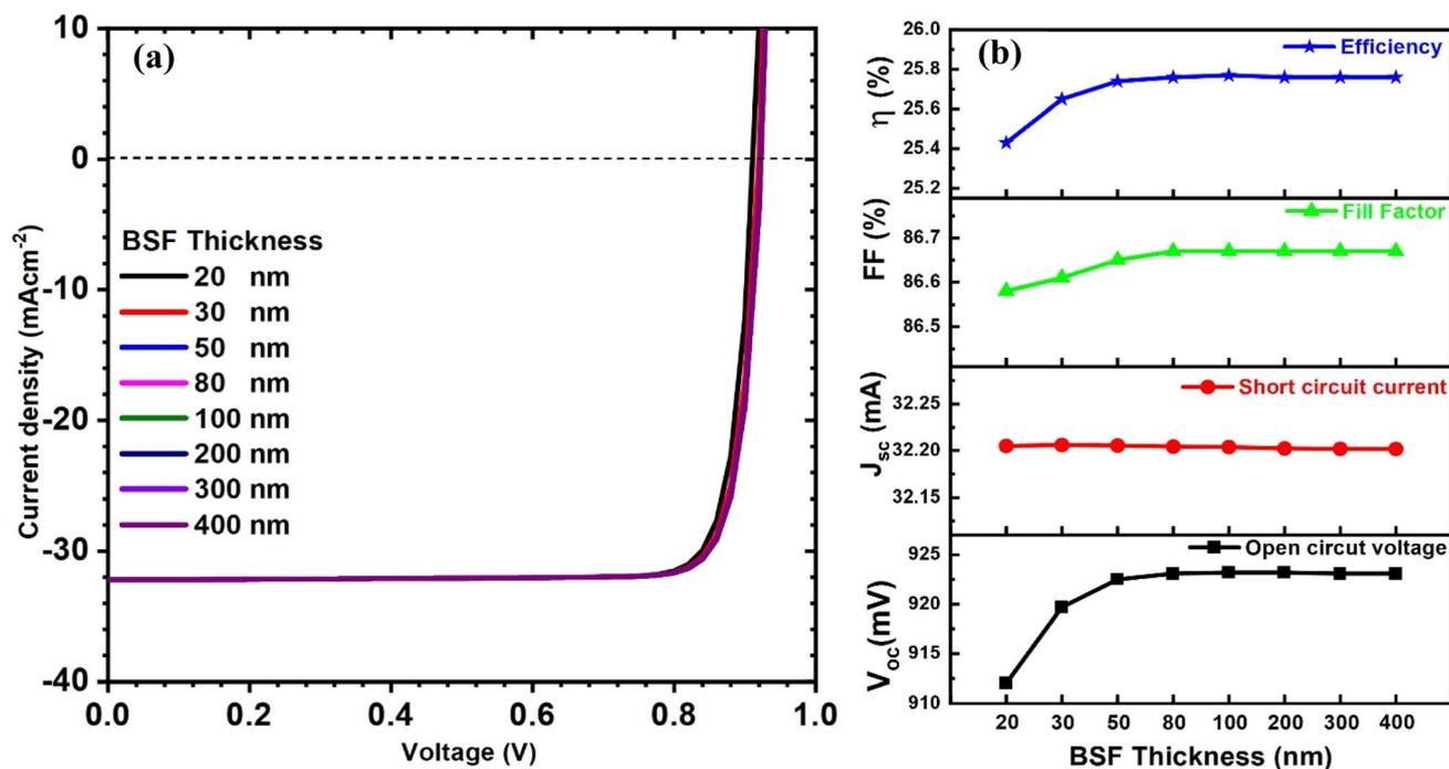
Fig. 10 Schematic of (a) current–voltage curves and (b) curves of PV parameters for CIGAS solar cells at different BSF thicknesses.
