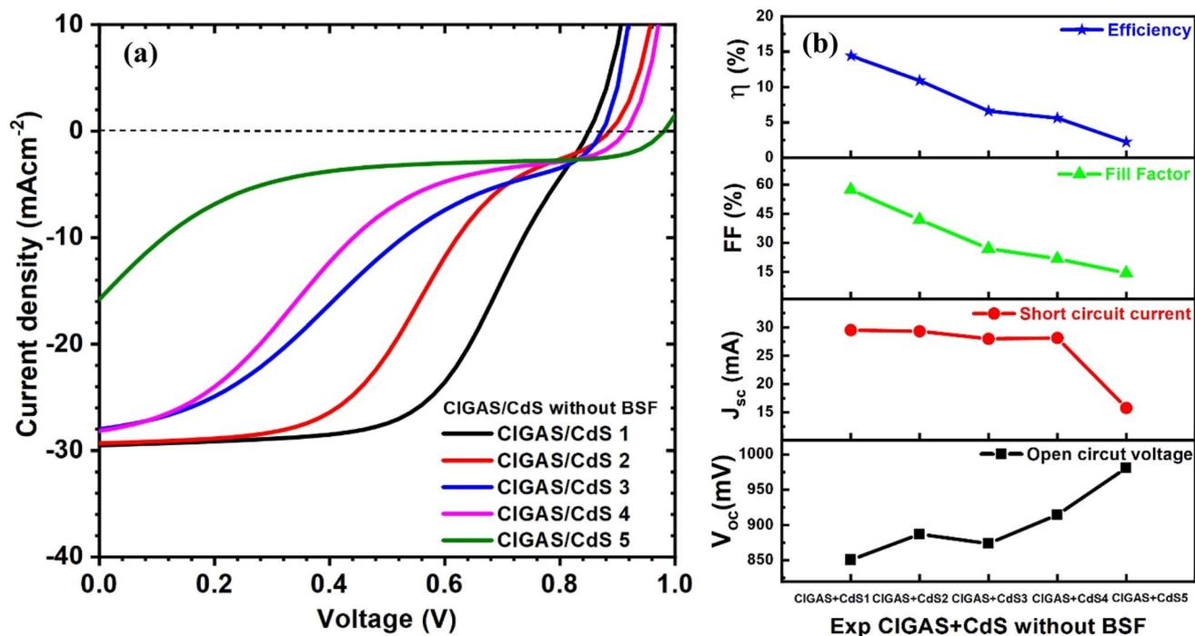
Fig. 17 Schematic of (a) current–voltage curves and (b) curves of PV parameters for CIGAS solar cells, fitting experimental parameters for CIGAS and CdS without BSF materials.
