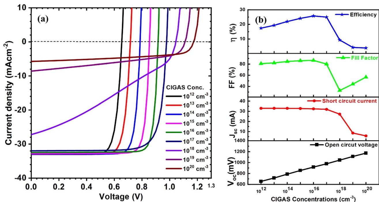
Fig. 4 Schematic of (a) current–voltage curves and (b) curves of PV parameters for CIGAS solar cells at CIGAS carrier concentrations ranging from 10<sup>12</sup> to 10<sup>20</sup> cm<sup>-3</sup>.
