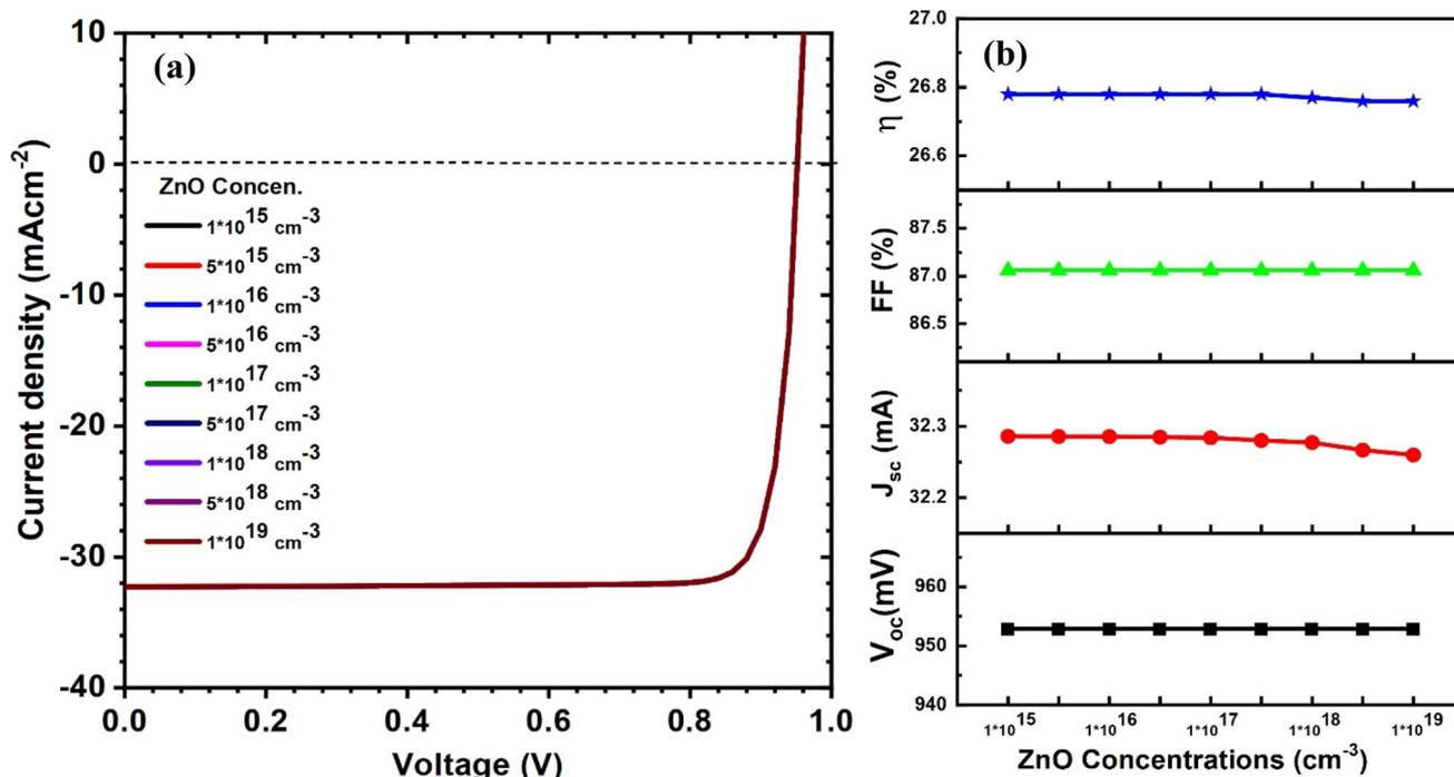
Fig. 9 Schematic of (a) current–voltage curves and (b) curves of PV parameters for CIGAS solar cells at different ZnO concentrations.
