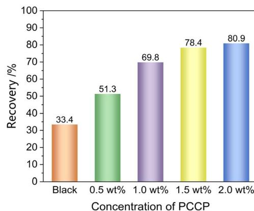
Fig. 5 Rolling recovery rate of shale cuttings in PCCP solutions with different concentrations.
