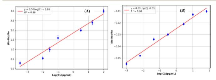
Fig. 10 (A) Calibration curve obtained by electrochemical impedance spectroscopy of the MIP, and (B) calibration curve by electrochemical impedance spectroscopy of the non-imprinted polymer.
