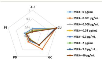
Fig. 13 Radar plots of the voltammetric electronic tongue responses toward the eight different milk samples (expressed as the difference between anodic and cathodic current peaks voltammograms).
