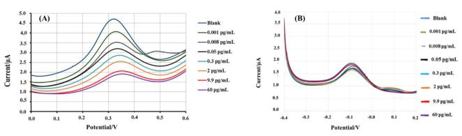
Fig. 7 (A) Cyclic voltammograms of the detection of tobramycin by the molecularly imprinted polymer sensor, and (B) cyclic voltammograms for the detection of tobramycin by the non-imprinted polymer sensor.
