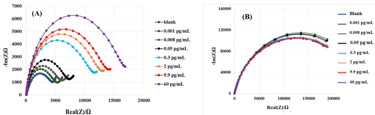
Fig. 9 (A) Nyquist diagrams of tobramycin detection by molecularly imprinted polymers sensor, and (B) Nyquist diagrams of tobramycin detection by the non-imprinted polymer sensor.
