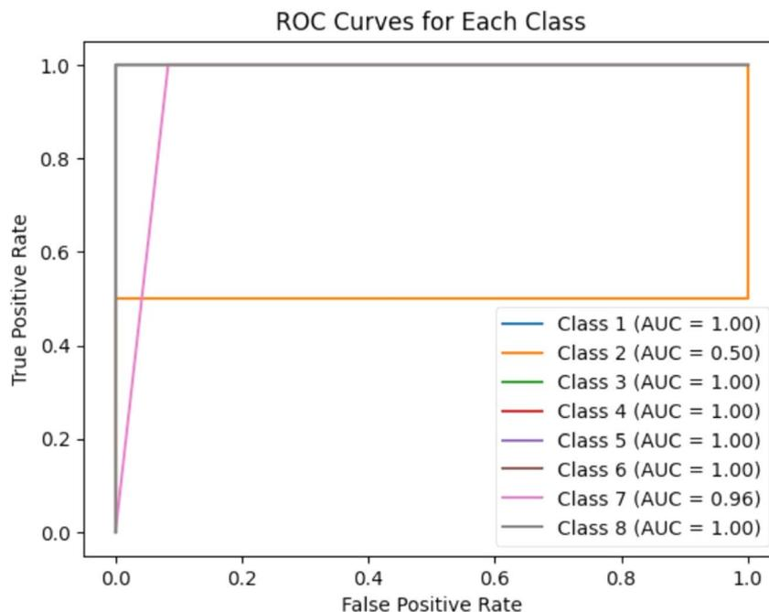
Fig. 16 Receiver operating characteristic curve displaying data points for eight different milk samples with data collected from the voltammetric electronic tongue.
