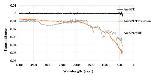
Fig. 3 Fourier transform infrared spectroscopy spectra obtained for bare gold, after molecularly imprinted polymer deposit, and after extraction.
