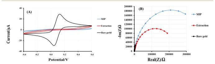
Fig. 6 (A) Cyclic voltammograms of the different stages of molecularly imprinted polymer sensor development, and (B) Nyquist diagrams of different stages in the development of the molecularly imprinted polymer sensor.
