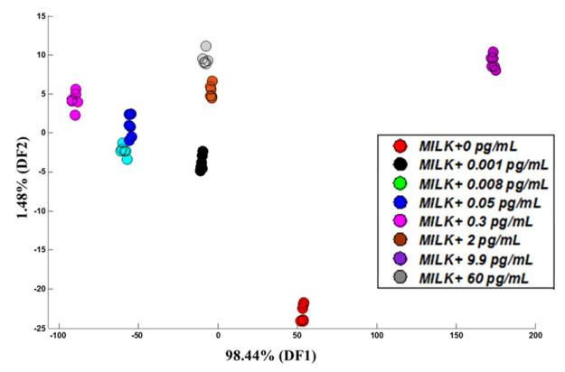
Fig. 15 Discriminant function analysis plot analysis using  $\Delta l$  and Area as features of the voltammetric electronic tongue system responses.
