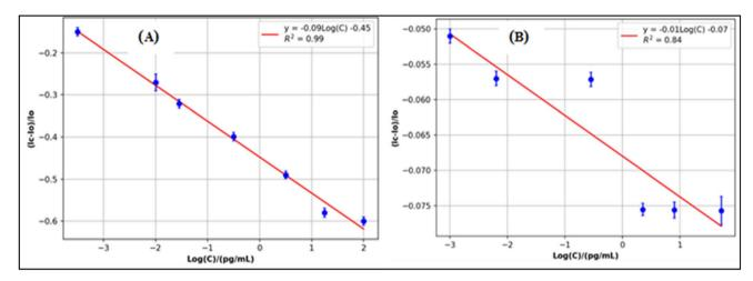
Fig. 8 (A) Differential pulse voltammetry calibration curve of molecularly imprinted polymers sensor, and (B) differential pulse voltammetry calibration curve of non-imprinted polymer sensor.
