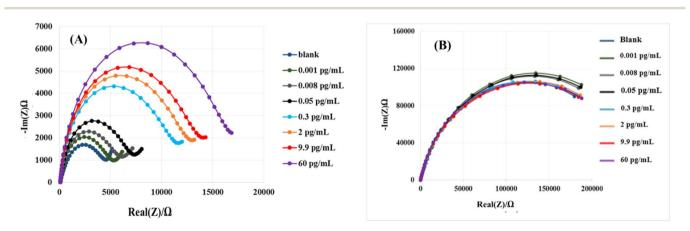
Fig. 9 (A) Nyquist diagrams of tobramycin detection by molecularly imprinted polymers sensor, and (B) Nyquist diagrams of tobramycin detection by the non-imprinted polymer sensor.
