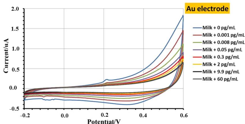
Fig. 12 Mean responses of the voltammetric electronic tongue gold electrode when exposed to eight different milk samples.
