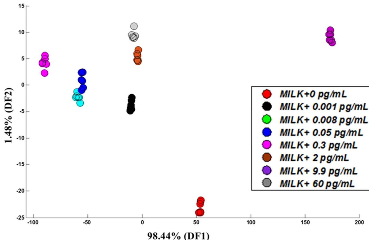
Fig. 15 Discriminant function analysis plot analysis using  $\Delta I$  and Area as features of the voltammetric electronic tongue system responses.
