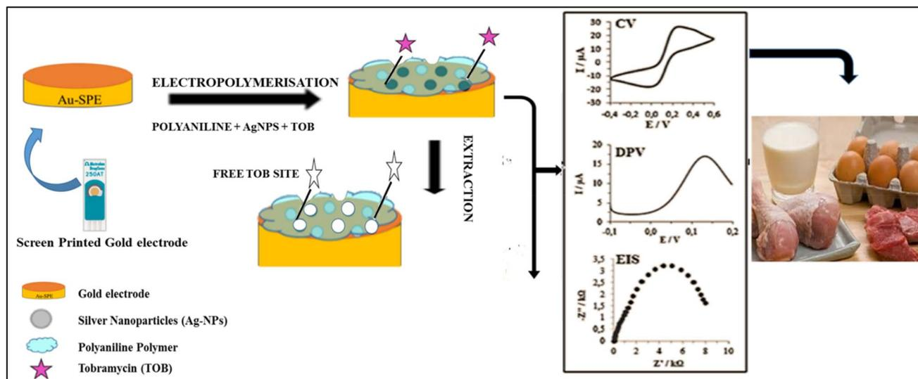
Fig. 1 Manufacturing process of the molecularly imprinted polymer sensor.
