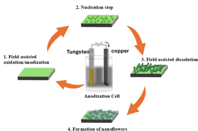
Fig. 8 The formation process of \text{WO}_3 nanoflowers on W sheet in \text{HNO}_3 based electrolyte via anodization.
