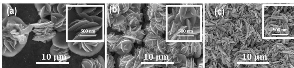
Fig. 6 Top surface FESEM morphology of  $\text{WO}_3$  nanoflowers obtained at 15 V for 15 min and at 90 °C at various  $\text{HNO}_3$  electrolyte concentrations (a) 0.5, (b) 1.5 M, and (c) 3.0 M with high-magnification images in the inset.
