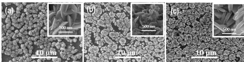
Fig. 5 Top surface FESEM morphology of  $\text{WO}_3$  nanoflowers obtained in 1.5 M  $\text{HNO}_3$  at 15 V, and 90 °C at different anodization duration (a) 15 min, (b) 30 min, and (c) 60 min with high magnification images in the inset.
