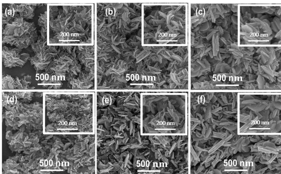
Fig. 4 FSEM images (a–c) of the top surfaces of the as-anodized  $\text{WO}_3$  nanostructures obtained at 15 V for 15 min at (a) 50, (b) 70, and (c) 90 °C, whereas the FESEM images of the respective annealed samples are given (d–f). The inset shows the respective high-magnification images.
