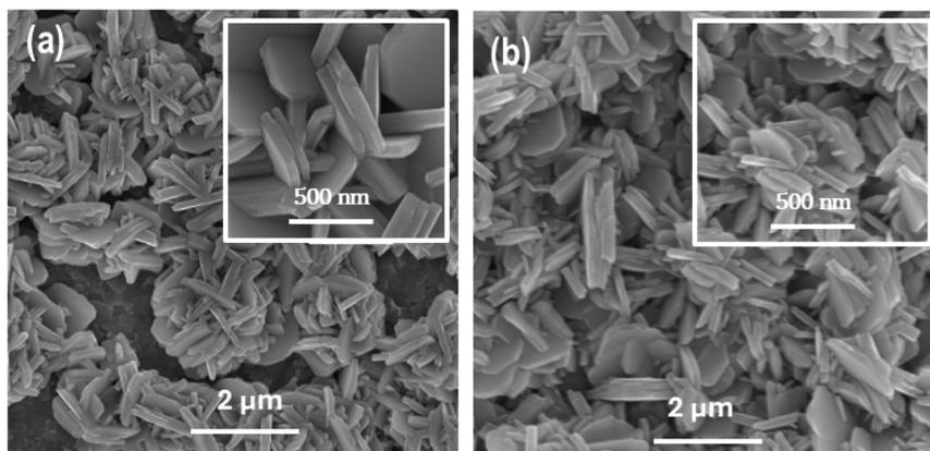
Fig. 7 Top surface FESEM morphology of  $\text{WO}_3$  nanostructure obtained in 1.5 M  $\text{HNO}_3$  at 15 V, 15 min, and 90 °C (a) without stirring and (b) with continuous stirring. The inset shows the high magnification images.
