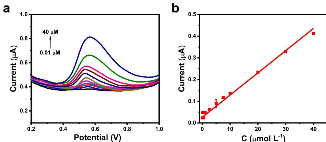
Fig. 6 DPVs for various BPA concentrations in 0.1 M phosphate buffer (pH = 7.0) at the GO/FeVO<sub>4</sub> sensor (a). Linear relationships between the oxidation peak currents and the concentrations of BPA (b).
