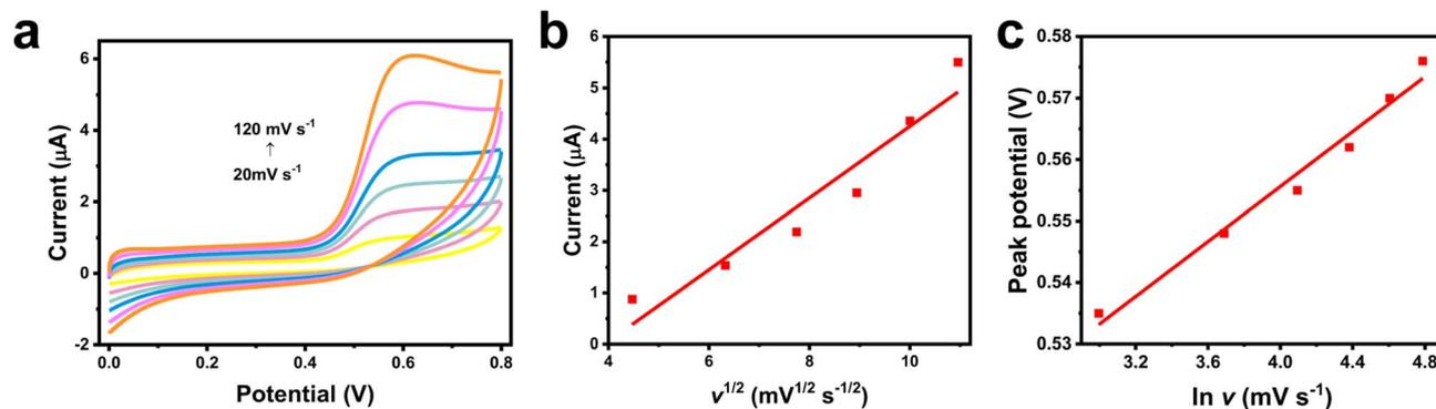
Fig. 5 CVs (a) of 20  $\mu\text{M}$  BPA detected by the GO/FeVO<sub>4</sub> electrode in 0.1 M phosphate buffer (pH = 7.0) at different scan rate from 20 to 120  $\text{mV s}^{-1}$ . The correlation between peak currents ( $I_{\text{pa}}$ ) and  $v^{1/2}$  ( $\text{mV}^{1/2} \text{s}^{-1/2}$ ) (b). The correlation of peak potential and Napierian logarithm of scan rate ( $\ln v$ ) (c).
