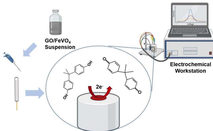
Scheme 1 The GO/FeVO<sub>4</sub> electrochemical sensor for BPA detection.
