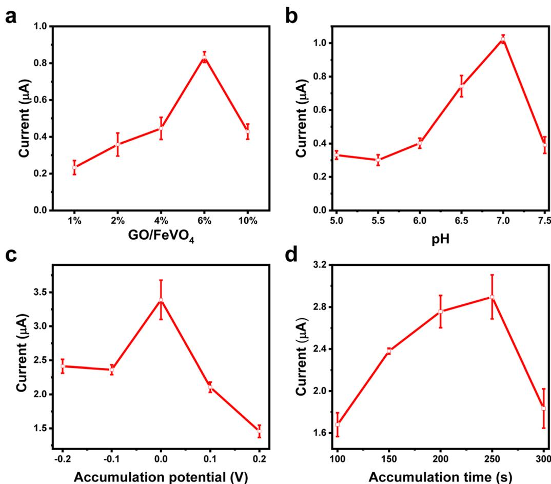
Fig. 4 The impact of various weight ratios of GO/ $\text{FeVO}_4$  (a), pH value (b), accumulation potential (c), and accumulation time (d) on the 20  $\mu\text{M}$  BPA peak current in 0.1 M phosphate buffer (pH = 7.0) was studied using the GO/ $\text{FeVO}_4$  sensor.
