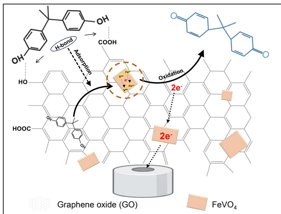
Scheme 2 BPA detection reaction mechanism at the GO/FeVO<sub>4</sub> sensor.
