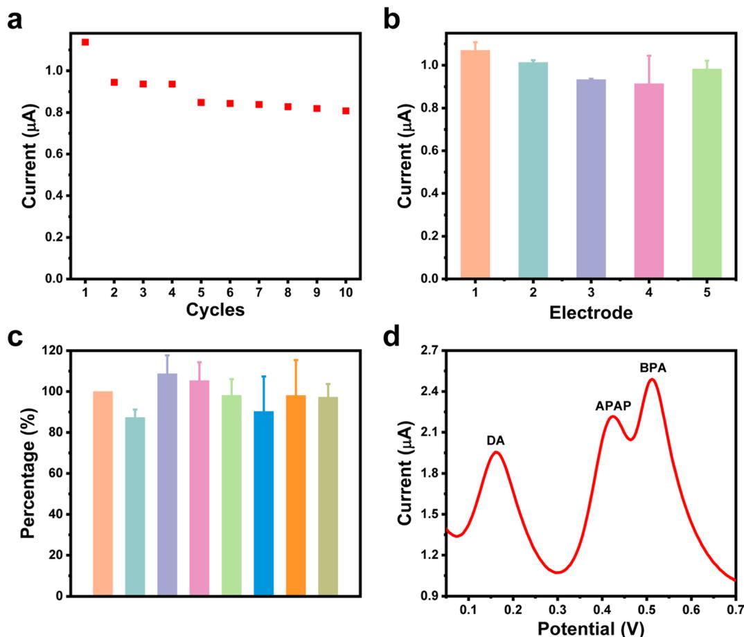
Fig. 7 The stability (a), reproducibility (b), anti-interference (c) and selectivity (d) of the GO/FeVO<sub>4</sub> sensor in 0.1 M phosphate buffer (pH = 7.0).
