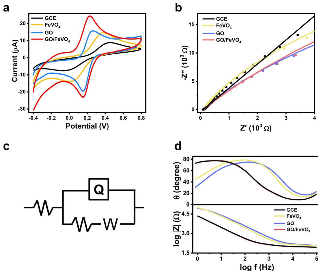
Fig. 2 CVs (a), Nyquist plots (b), equivalent circuit (c) and Bode plots (d) of GCE, FeVO<sub>4</sub>, GO and GO/FeVO<sub>4</sub> in a 2.5 mM K<sub>3</sub>[Fe(CN)<sub>6</sub>]/K<sub>4</sub>[Fe(CN)<sub>6</sub>] solution containing 0.1 M KCl. Equivalent circuit was used for simulating EIS.
