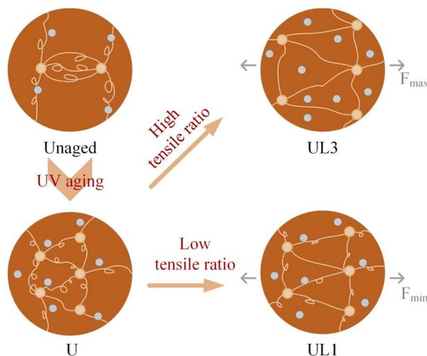
Fig. 15 States of molecular chains of HTV-SR and fillers under UV and tensile effects.
