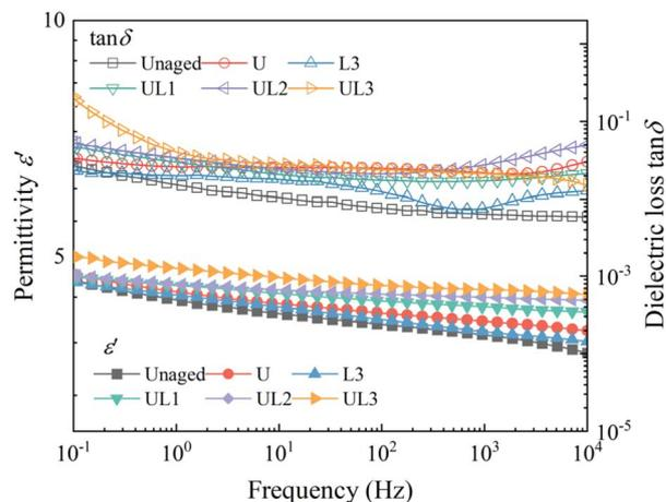
Fig. 12 Dielectric spectra of HTV-SR samples under different aging conditions.
