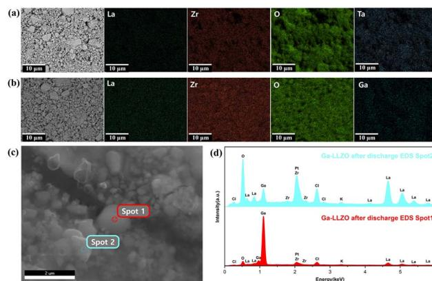
Fig. 4 Top-view SEM images with corresponding EDS elemental mapping of pristine (a) Ta-doped LLZO and (b) Ga-doped LLZO pellets. (c) Cross-sectional SEM image of Ga-doped LLZO disk after the thermal battery discharge test and (d) EDS spectra of Spots 1 and 2.
