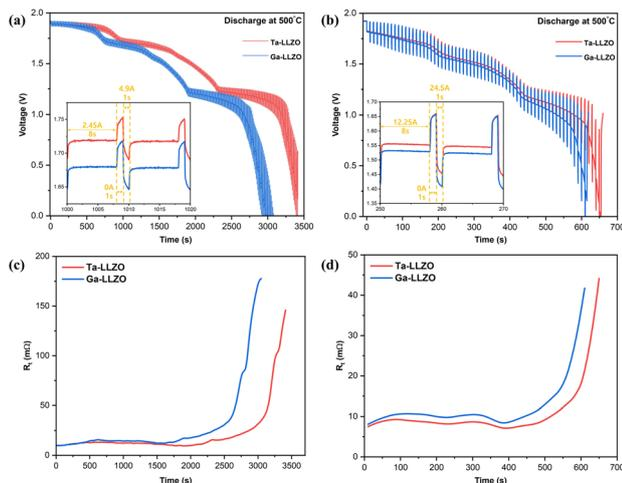
Fig. 2 Thermal battery discharge test results of Ta- and Ga-doped LLZO under constant current densities of (a)  $0.1 \text{ A}_{\text{avg}} \text{ cm}^{-2}$  and (b)  $0.5 \text{ A}_{\text{avg}} \text{ cm}^{-2}$ . Internal resistance over time according to discharge curves derived from Ohm's law at (c)  $0.1 \text{ A}_{\text{avg}} \text{ cm}^{-2}$  and (d)  $0.5 \text{ A}_{\text{avg}} \text{ cm}^{-2}$ .
