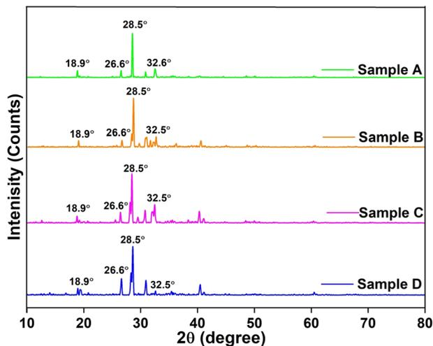
Fig. 7 XRD plots for char obtained from microwave-assisted co-pyrolysis of biomass and plastic.
