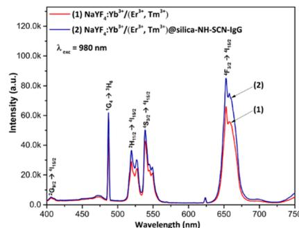
Fig. 5 UCPL spectra of  $\text{NaYF}_4:\text{Yb}^{3+}/(\text{Er}^{3+}, \text{Tm}^{3+})$  (1) and  $\text{NaYF}_4:\text{Yb}^{3+}/(\text{Er}^{3+}, \text{Tm}^{3+})@$ silica-NH-SCN-IgG nanoparticles (2) under 980 nm excitation.
