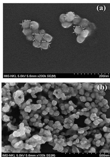
Fig. 1 FESEM images of  $\text{NaYF}_4:\text{Yb}^{3+}/(\text{Er}^{3+},\text{Tm}^{3+})$  nanoparticles: (a) high-magnification image at 200 nm scale and (b) lower magnification image at 500 nm scale, respectively.
