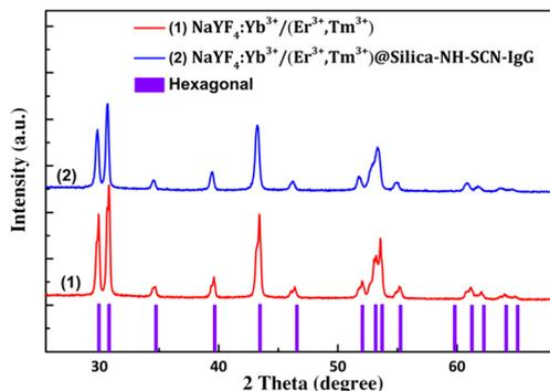
Fig. 3 X-ray diffraction patterns of the (1)  $\text{NaYF}_4:\text{Yb}^{3+}/(\text{Er}^{3+}, \text{Tm}^{3+})$  and (2)  $\text{NaYF}_4:\text{Yb}^{3+}/(\text{Er}^{3+}, \text{Tm}^{3+})@$ silica-NH-SCN-IgG nanoparticles.
