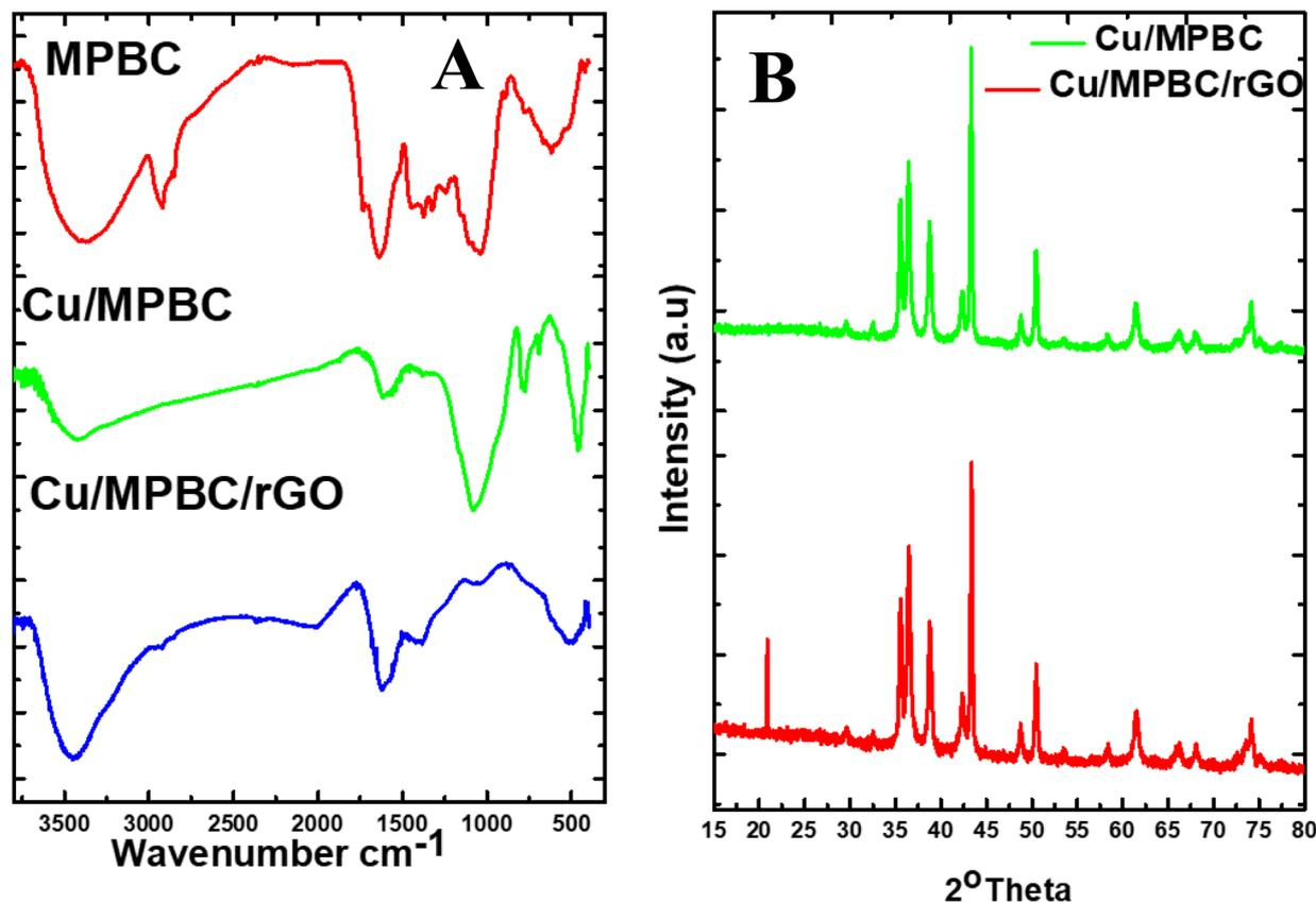
Fig. 1 (A). Fourier-transformed infrared spectroscopy spectra, (B) X-ray diffraction patterns of Cu/MPBC and Cu/MPBC/rGO.
