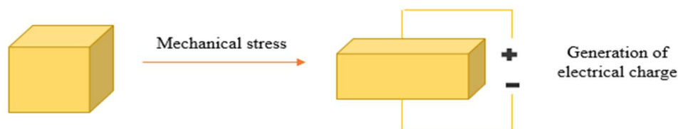
(A) Mechanical Stress-Induced Response in Piezoelectric Materials
