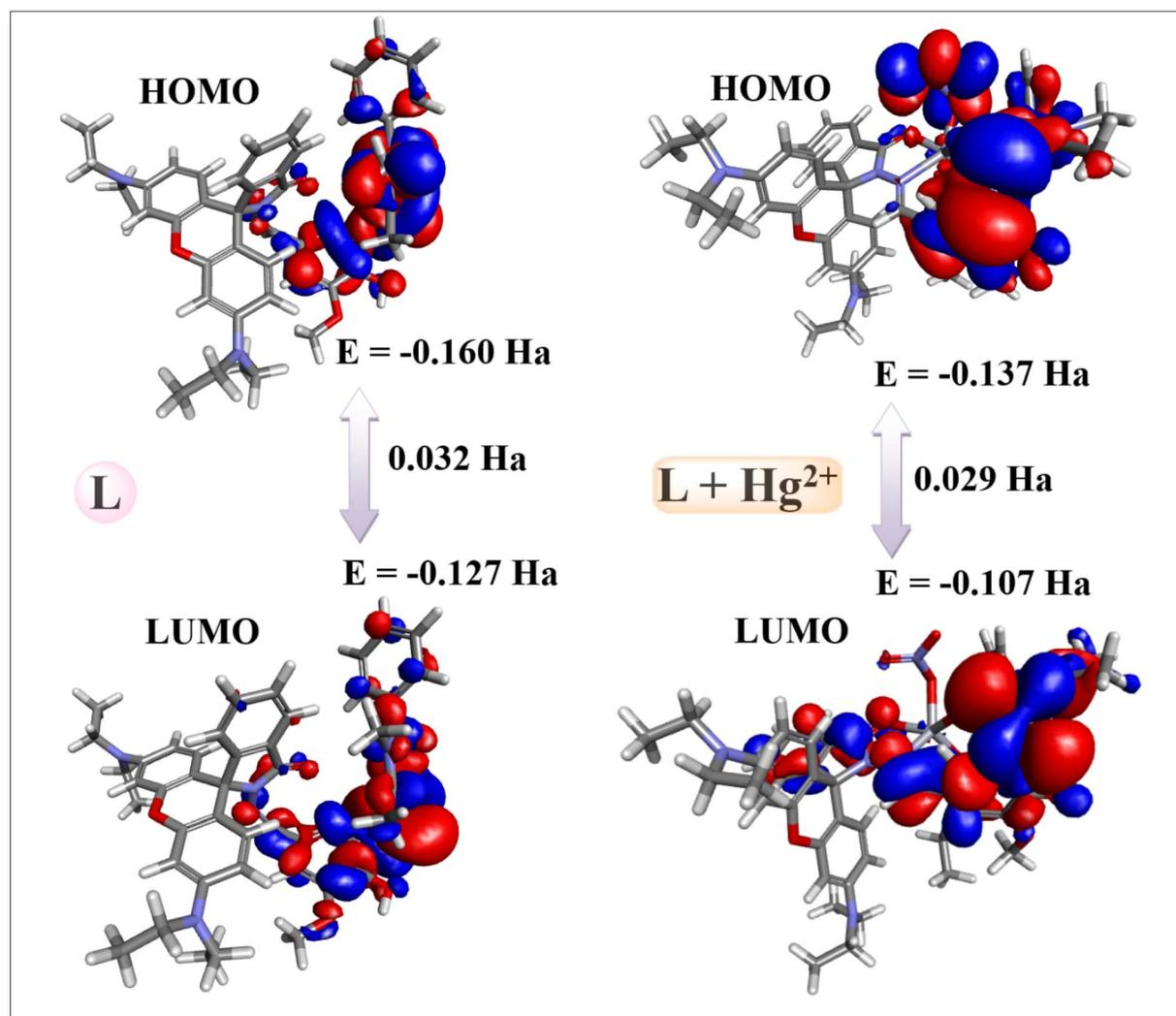
Fig. 14 HOMO and LUMO orbitals and along with their energies in L and L + Hg<sup>2+</sup>.
