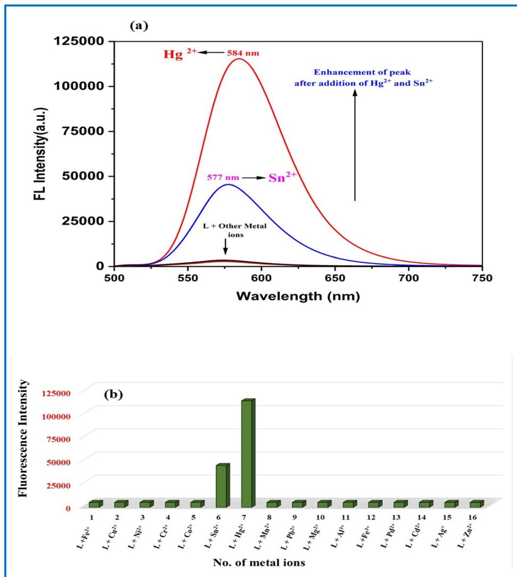
Fig. 7 (a) Emission spectral nature of L (20 μM) upon addition of various metal ions (Fe<sup>2+</sup>, Cu<sup>2+</sup>, Ni<sup>2+</sup>, Cr<sup>2+</sup>, Co<sup>2+</sup>, Sn<sup>2+</sup>, Hg<sup>2+</sup>, Mn<sup>2+</sup>, Pb<sup>2+</sup>, Mg<sup>2+</sup>, Al<sup>3+</sup>, Fe<sup>3+</sup>, Pd<sup>2+</sup>, Cd<sup>2+</sup>, Ag<sup>+</sup> and Zn<sup>2+</sup>) in a HEPES buffer (b) column plot for the emission spectral intensity of L (50 μM) upon addition of different metal ions.
