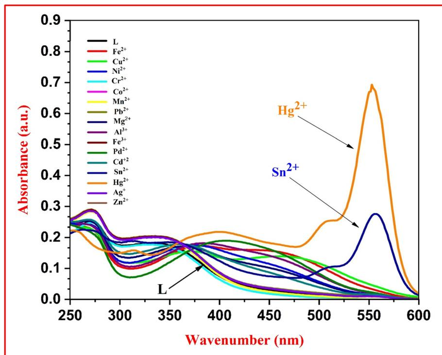
Fig. 1 UV-Vis spectra of L (40  $\mu$ M) upon addition of various metal ions (Fe<sup>2+</sup>, Cu<sup>2+</sup>, Ni<sup>2+</sup>, Cr<sup>2+</sup>, Co<sup>2+</sup>, Sn<sup>2+</sup>, Hg<sup>2+</sup>, Mn<sup>2+</sup>, Pb<sup>2+</sup>, Mg<sup>2+</sup>, Al<sup>3+</sup>, Fe<sup>3+</sup>, Pd<sup>2+</sup>, Cd<sup>2+</sup>, Ag<sup>+</sup> and Zn<sup>2+</sup>) in a HEPES buffer [C<sub>2</sub>H<sub>5</sub>OH-H<sub>2</sub>O (4 : 1, v/v) pH = 7.2] at 25 °C.
