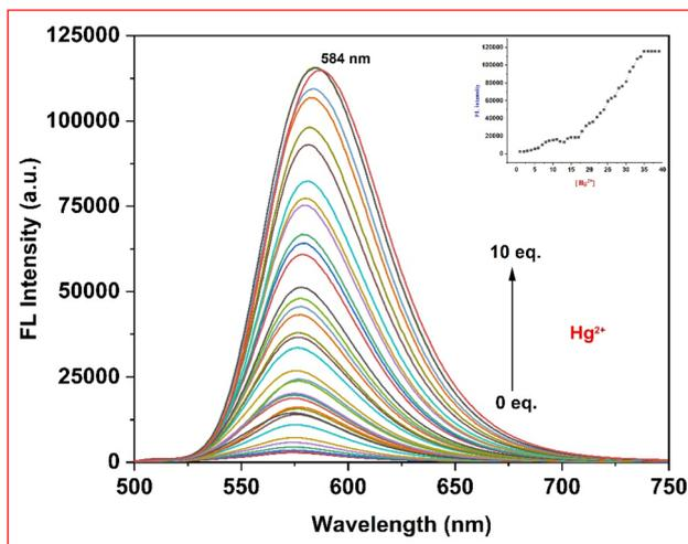
Fig. 8 (a) Changes in the emission spectrum of L (40  $\mu\text{M}$ ) at 25  $^{\circ}\text{C}$  after the addition of the  $\text{Hg}^{2+}$  ion in a HEPES buffer [50  $\mu\text{M}$ ,  $\text{C}_2\text{H}_5\text{OH}-\text{H}_2\text{O}$  (4 : 1, v/v, pH = 7.2)] [ $\text{Hg}^{2+}$ ] = 0–10 eq. (b) Inset: 584 nm intensity vs. the quantity of equivalent  $\text{Hg}^{2+}$  added.
