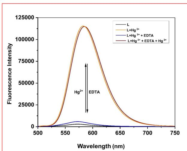
Fig. 9  $\text{Hg}^{2+}$  complex of L (40  $\mu\text{M}$ ) emission spectrum changes when EDTA is added in a HEPES buffer solution [50  $\mu\text{M}$ ,  $\text{C}_2\text{H}_5\text{OH}-\text{H}_2\text{O}$  (4 : 1, v/v, pH = 7.2)] at 25  $^{\circ}\text{C}$ . EDTA = 0–10 eq.
