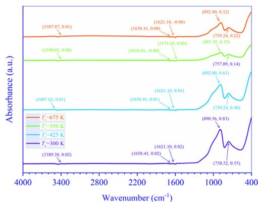
Fig. 7 FTIR spectra of  $T_s$  modified CdIn<sub>2</sub>Se<sub>4</sub> thin films.
