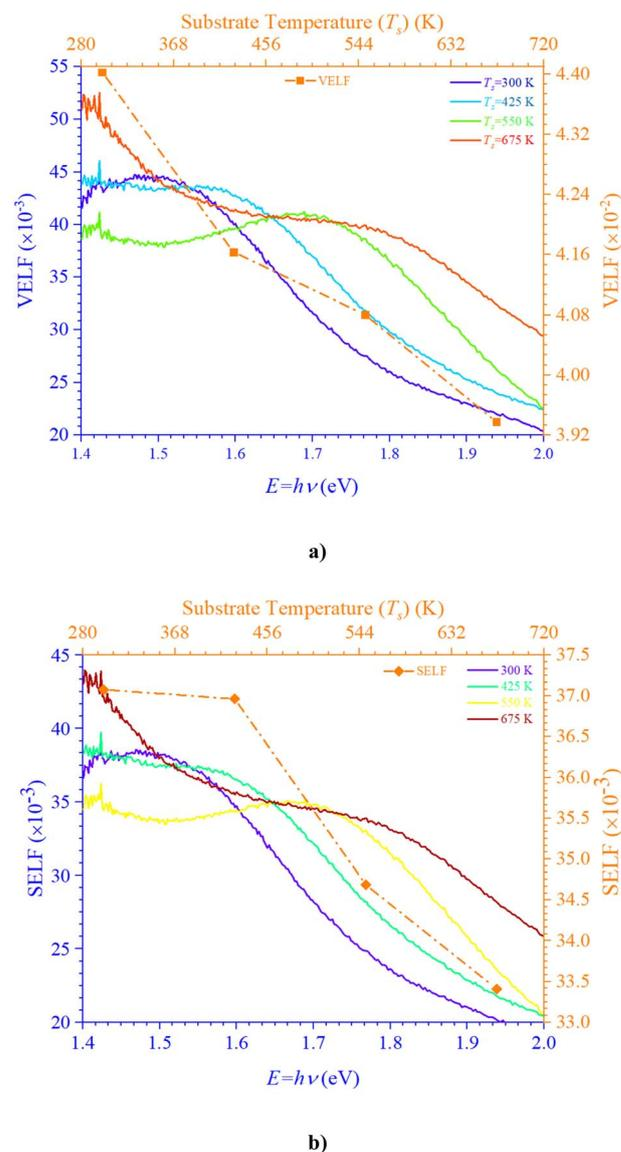
Fig. 6 Variation in (a) VELF and (b) SELF of CdIn<sub>2</sub>Se<sub>4</sub> thin films as a function of energy.
