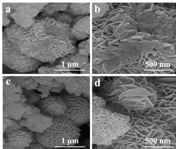
Fig. 2 SEM images of NiFe-V<sub>0</sub> (a and b) and NiFe-V<sub>1.0</sub> (c and d).
