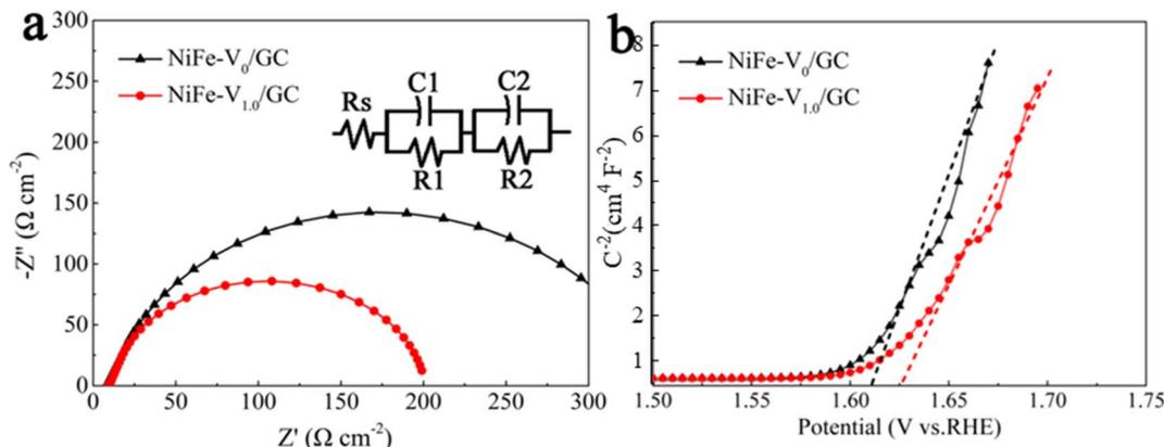
Fig. 10 Nyquist curves and the equivalent circuits for NiFe-V<sub>0</sub>/GCE and NiFe-V<sub>1.0</sub>/GCE measured at open-circuit potential (OCP = 0.35 V vs. RHE) (a), Mott-Schottky curves (b).
