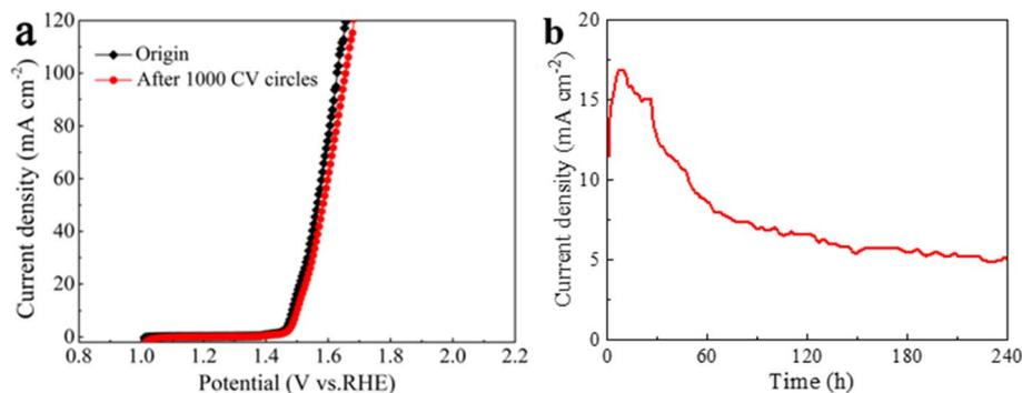
Fig. 8 (a) LSV curves and (b) chronoamperometric test of the NiFe-V<sub>1.0</sub>/CCF electrode.
