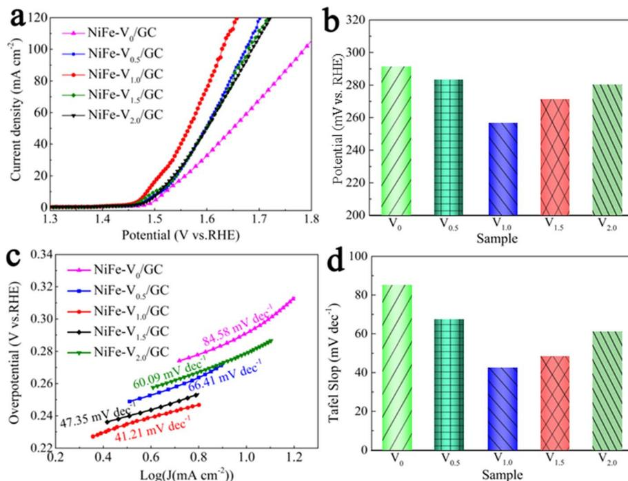
Fig. 7 LSV curves of different NiFe-V<sub>x</sub>/GCE samples (a), OER overpotential histograms (b) at 10 mA cm<sup>-2</sup> corresponding to (a); Tafel curves (c), Tafel slope histograms (d) corresponding to (c).
