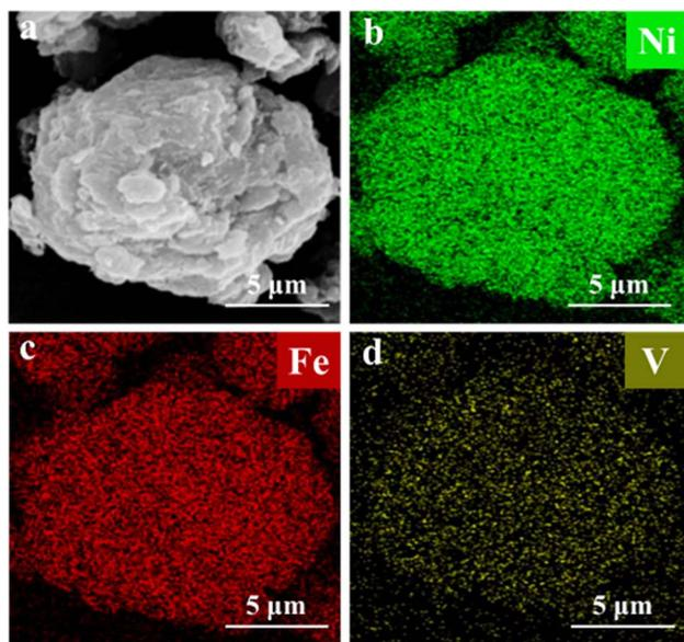
Fig. 3 (a) EDS spectrum and (b–d) corresponding elemental mapping images of NiFe-V<sub>1.0</sub>, confirming the uniform distribution of Ni, Fe and V.
