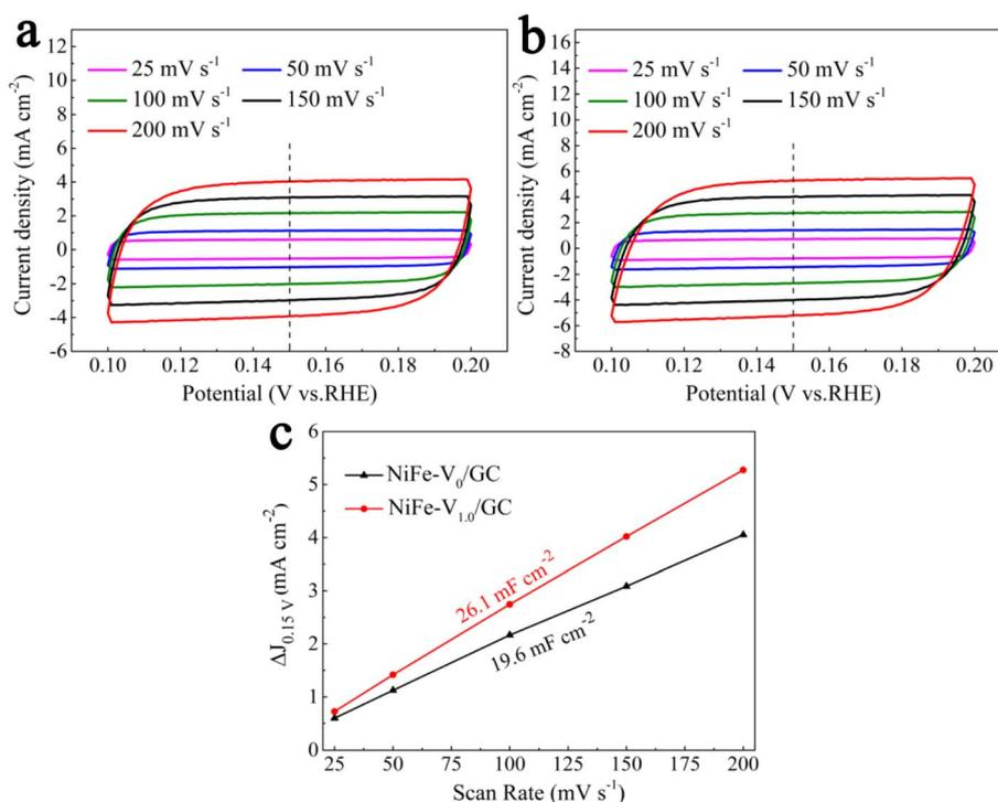
Fig. 9 CV curves of NiFe-V<sub>0</sub>/GCE (a) and NiFe-V<sub>1.0</sub>/GCE (b) at 25–200 mV s<sup>-1</sup> scan rates;  $C_{dl}$  and electrochemical activity surface area (c) specific capacitance (0.5 $\Delta j/v$ ) versus scan rate.
