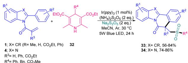
Scheme 11 Ir-catalyzed sulfonylation/cyclization of *N*-acryloyl 2-aryl benzimidazole/indole with Hantzsch esters and  $\text{Na}_2\text{S}_2\text{O}_5$ .
