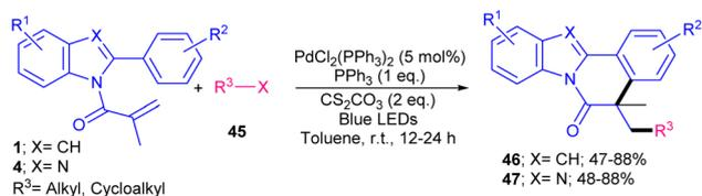
Scheme 17 Pd-catalyzed alkylation/cyclization of *N*-methacryloyl 2-phenyl indoles/benzimidazoles.
