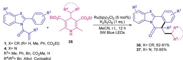
Scheme 12 Ru-catalyzed alkylation/cyclization of *N*-methacryloyl 2-phenyl benzimidazoles/indoles.
