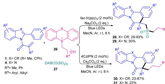
Scheme 10 Ir-catalyzed sulfonylation/cyclization of *N*-methacryloyl 2-phenyl benzimidazoles/indoles with DABCO ( $\text{SO}_2$ )<sub>2</sub> and thianthrenium salts.
