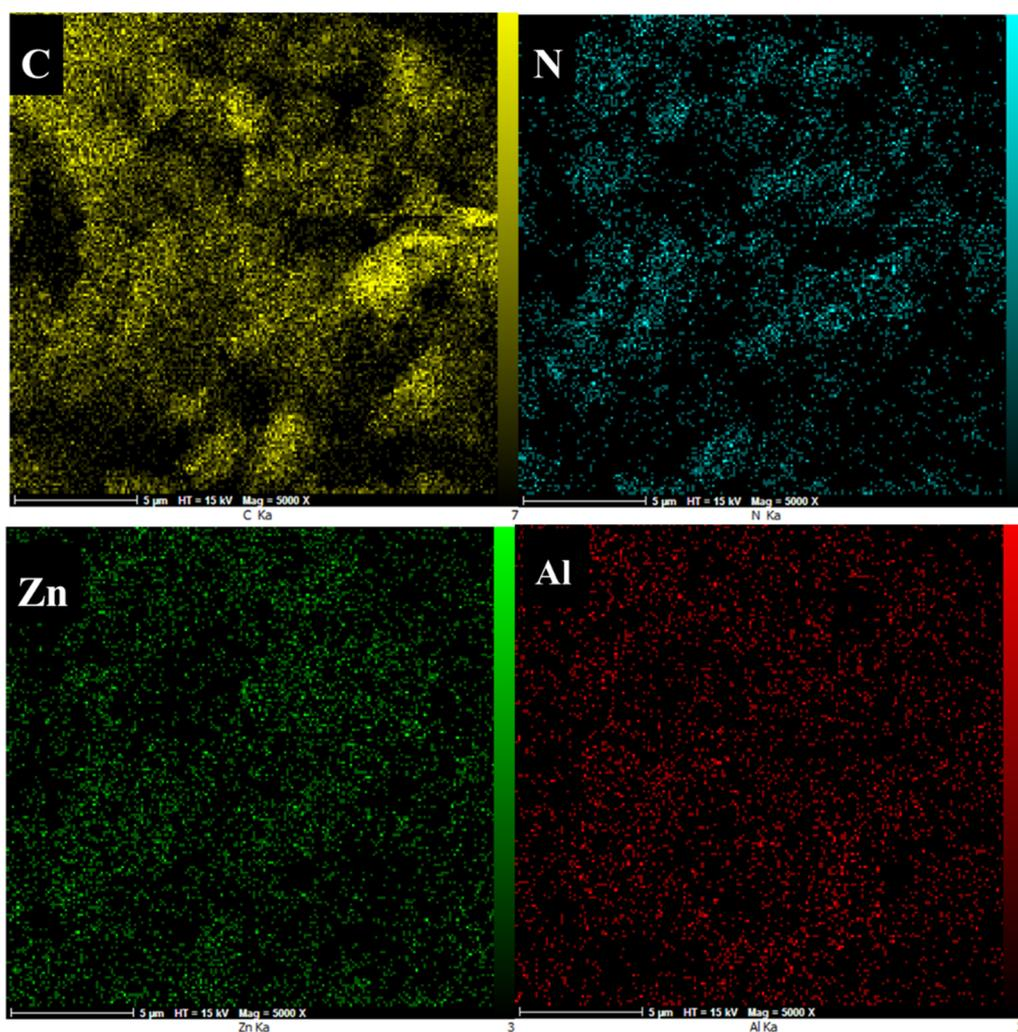
Fig. 6 Elemental mapping of COP@ZIF-8.
