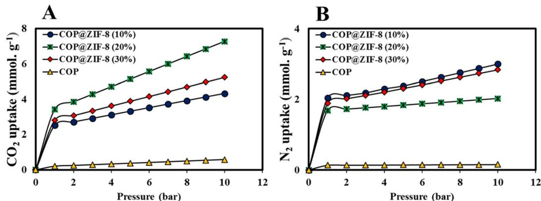
Fig. 11 (A) CO<sub>2</sub> adsorption, and (B) N<sub>2</sub> adsorption of COP and COP@ZIF-8 (10–30%) at 300.15 K and up to 1–10 bar.
