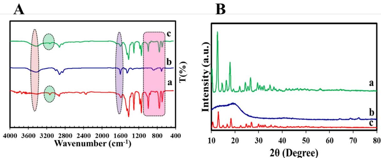
Fig. 3 (A) FT-IR results of (a) ZIF-8 NPs, (b) COP, (c) COP@ZIF-8; (B) XRD of (a) ZIF-8 NPs, (b) COP, (c) COP@ZIF-8.
