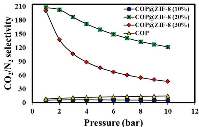
Fig. 12 IAST predicted selectivity for CO<sub>2</sub>/N<sub>2</sub> (15 : 85) of COP@ZIF-8 core-shell.
