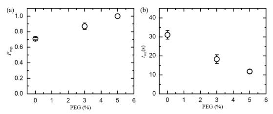
Fig. 6 PEG-DOPE% dependent probability of rupture and average survival time of GUVs at  $\sigma_c = 5$  mN m<sup>-1</sup>. (a) Probability of rupture and (b) average survival time. Error bar represents the standard deviation (SD) obtained from 3–5 independent experiments.
