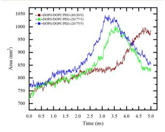
Fig. 10 Variation in SASA with time during electroporation in the DOPC/DOPG/PEG-DLGL bilayer at a constant DC electric field of 0.4 V nm<sup>-1</sup>.
