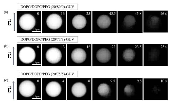
Fig. 4 Fluorescence microscopic image of rupture of a (a) DOPG/DOPC/PEG-DOPE (20/80/0)-GUV (b) DOPG/DOPC/PEG-DOPE (20/77/3)-GUV, and (c) DOPG/DOPC/PEG-DOPE (20/75/5)-GUV under  $\sigma_c = 5$  mN m $^{-1}$ . The arrow on the left side indicates the electric field direction. The numbers in each image indicate the time in seconds.
