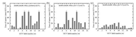
Fig. 5 Stochastic rupture time of several 'single GUVs' at  $\sigma_c = 5 \text{ mN m}^{-1}$  containing (a) 0% PEG-DOPE, (b) 3% PEG-DOPE, and (c) 5% PEG-DOPE in their membranes. The ( $\times$ ) mark at the top of the bar indicates that the GUV did not rupture within 60 s.
