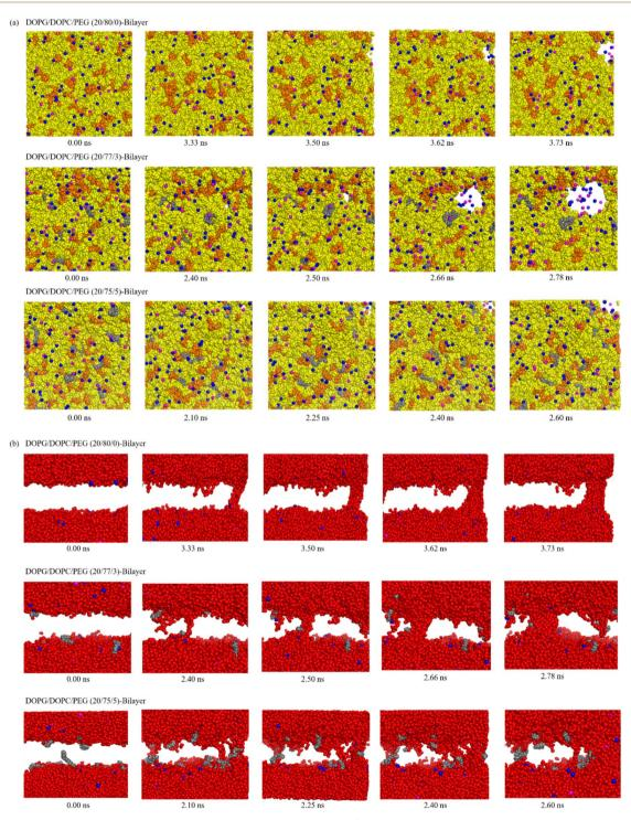
Fig. 8 Dynamics of pore formation by a constant DC electric field of  $0.4 \,\mathrm{V}\,\mathrm{nm}^{-1}$  in the DOPC/DOPG/PEG-DLGL bilayer. (a) Top view of the lipid bilayer, where the yellow, orange, and gray spheres indicate the DOPC, DOPG, and PEG-DLGL lipids, respectively. Blue and magenta spheres indicate the Na $^+$  and Cl $^-$  ions, respectively. (b) Side view of water molecules inside and outside the lipid bilayer (blank space), which is hidden.
