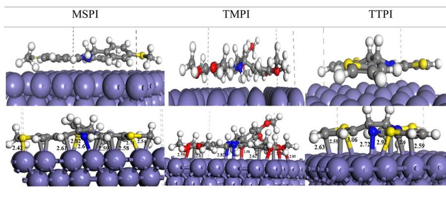
Fig. 17 Optimized adsorption geometries of **MSPI**, **TMPI**, and **TTPI** molecules on the Fe (110) surface as determined by *ab initio* DFT simulations.
