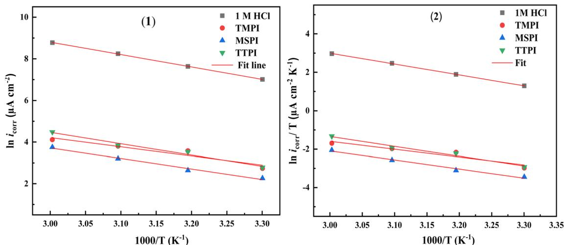
Fig. 6 Arrhenius (1) and transition state (2) plots of carbon steel in 1 M HCl solution without and with  $10^{-3}$  M of dihydroimidazoles at various temperatures.
