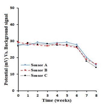
Fig. 5 Stability of MWCNT/Cu-PXM/MIP using 3 replicate sensors (A–C). Measurements were recorded in 1.0  $\times$  10<sup>-3</sup> M PXM.
