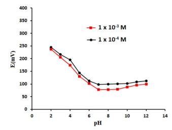
Fig. 7 Effect of pH on the response of MWCNT/Cu-PXM/MIP using the 1.0  $\times$  10<sup>-4</sup> M and 1.0  $\times$  10<sup>-3</sup> M PXM solutions [working pH range: 7–9]
