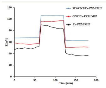
Fig. 6 Water layer test for MWCNT/Cu-PXM/MIP, GNC/Cu-PXM/MIP and Cu-PXM/MIP sensors. Measurements were recorded in 1.0  $\times$   $10^{-3}$  M PXM then 1.0  $\times$   $10^{-2}$  M perindopril and finally 1.0  $\times$   $10^{-3}$  M PXM.
