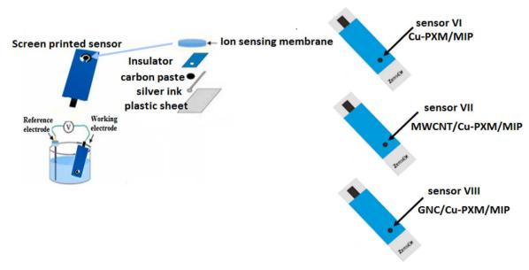
Fig. 2 Schematic representation of screen-printed electrodes (VI–VIII).
