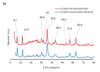
Fig. 1 (a) FT-IR spectra of as-synthesized Ni-MOF74, Ni-MOF74/ Fe $_3O_4$ /SiO $_2$ /NH $_2$ , Ni-MOF74/Fe $_3O_4$ /SiO $_2$ /NH $_2$ / $\beta$ -CD. (b) XRD powder pattern (inset shows the crystal structure of Ni-MOF74/Fe $_3O_4$ /SiO $_2$ /NH $_2$  and Ni-MOF74/Fe $_3O_4$ /SiO $_2$ /NH $_2$  and Ni-MOF74/Fe $_3O_4$ /SiO $_2$ /NH $_2$ / $\beta$ -CD).
