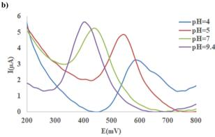
Fig. 4 SWAS voltammograms of 4-NP (30 ppm) at the Ni-MOF74/  $Fe_3O_4/SiO_2/NH_2/\beta$ -CD/GCE surface in the PBS (0.1 M) at different pH (4.00–9.40), scan rate 100 mv s<sup>-1</sup>,duration time120 s, pulse = 500 mV. (a) Experimental data, (b) pretreated data.
