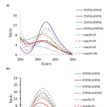
Fig. 9 (a) SWAS voltammograms of 2-NP (10 ppm) with 2-NP (10–100ppm); and (b) 2-NP (30 ppm) with 4-NP (10–100ppm) at the Ni-MOF74/Fe $_3O_4$ /SiO $_2$ /NH $_2$ / $\beta$ -CD/GCE surface in the PBS (0.1 M, pH = 9.40) at scan rate 100 and duration time 50 s, pulse = 500 mV.
