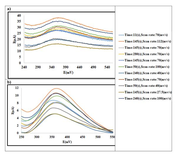
Fig. 5 SWAS voltammograms of 2-NP (60 ppm) at the Ni-MOF74/Fe<sub>3</sub>O<sub>4</sub>/SiO<sub>2</sub>/NH<sub>2</sub>/ $\beta$ -CD/GCE surface in the PBS (0.1 M, pH = 9.40) at different scan rate (27.5–112 mv s<sup>-1</sup>) and different duration time (11–240 s), pulse = 500 mV. Experimental data (a) and pretreated data (b).
