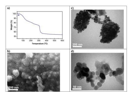
Fig. 2 Characterization of Ni-MOF74/Fe $_3$ O $_4$ /SiO $_2$ /NH $_2$ / $\beta$ -CD: (a) TGA plot (b) FE-SEM images (inset shows the magnified image), (c and d) TEM images.
