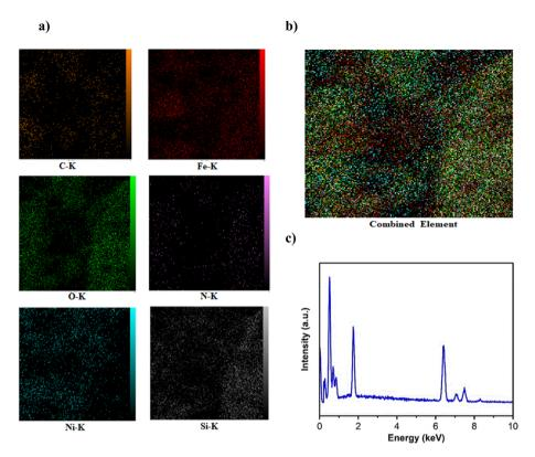
Fig. 3 EDX images of Ni-MOF74/Fe $_3$ O $_4$ /SiO $_2$ /NH $_2$ / $\beta$ -CD: (a) distribution of each involving element in the nanocomposite (indicated by different colors); (b) distribution for the combined elements; (c) EDX spectrum of the nanocomposite.
