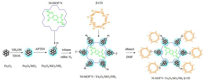
Scheme 1 Synthesis procedure of preparing Ni-MOF74/Fe<sub>3</sub>O<sub>4</sub>/SiO<sub>2</sub>/NH<sub>2</sub>/β-CD nanoparticles.
