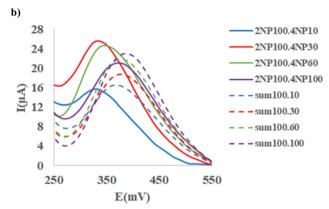
Fig. 10 (a) SWAS voltammograms of 2-NP (60 ppm) with 2-NP (10-100ppm); and (b) 2-NP (1000 ppm) with 4-NP (10-100ppm) at the Ni-MOF74/Fe<sub>3</sub>O<sub>4</sub>/SiO<sub>2</sub>/NH<sub>2</sub>/ $\beta$ -CD/GCE surface in the PBS (0.1 M, pH = 9.40) at scan rate 100 and duration time 50 s, pulse = 500 mV
