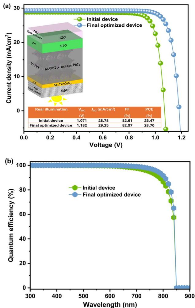
Fig. 11 (a)  $J$ - $V$  curves of initial and final optimized device with structure RGO/Se:Te/CuO<sub>2</sub>/MAPbI<sub>3</sub> + PbI<sub>2</sub> excess/STO/IZO. Inset presents structure and table summarizing all PV performance before and after optimization. (b) Quantum Efficiency (QE).
