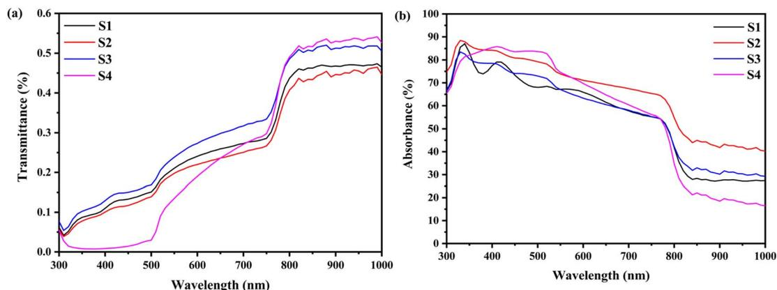
Fig. 4 (a) Optical transmittance spectra, (b) absorbance spectra of MAPbI<sub>3</sub> films with different DMF : DMSO ratios of samples S1, S2, S3 and S4.
