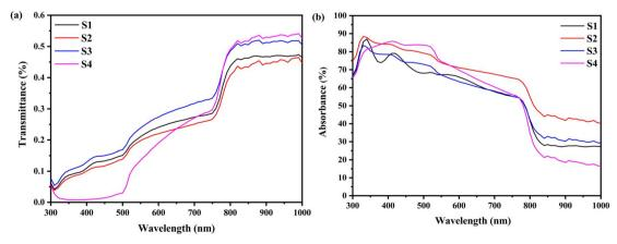
(a) Optical transmittance spectra, (b) absorbance spectra of MAPbl<sub>3</sub> films with different DMF: DMSO ratios of samples S1, S2, S3 and S4.
