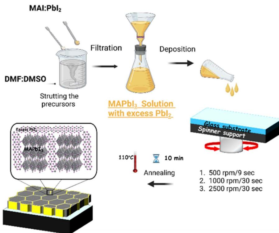
Fig. 2 Overview schematics of MAPbI<sub>3</sub> films fabrication procedures.
