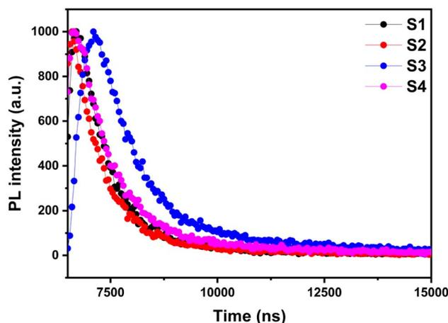
Fig. 6 TRPL spectra of MAPbI<sub>3</sub> films prepared with different DMF : DMSO ratios (S1, S2, S3 and S4).
