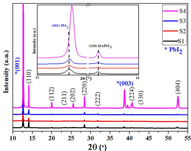
Fig. 3 X-ray diffraction spectra of perovskite layers for different DMF : DMSO ratios.
