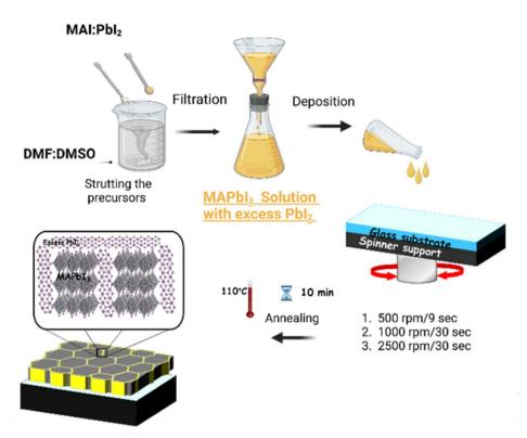
Fig. 2 Overview schematics of MAPbl<sub>3</sub> films fabrication procedures.
