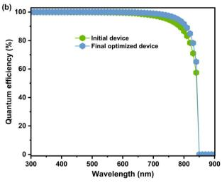
Fig. 11 (a) J-V curves of initial and final optimized device with structure RGO/Se:Te/CuO<sub>2</sub>/MAPbI<sub>3</sub> + PbI<sub>2</sub> excess/STO/IZO. Inset presents structure and table summarizing all PV performance before and after optimization. (b) Quantum Efficiency (QE).
