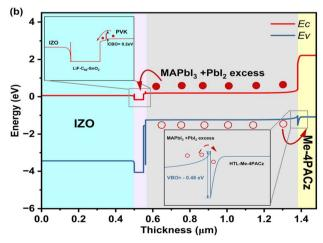
Fig. 7 (a) J-V curves, for all samples. Inset showing a table summarizing the PV parameters. (b) The band diagram of one of the samples.
