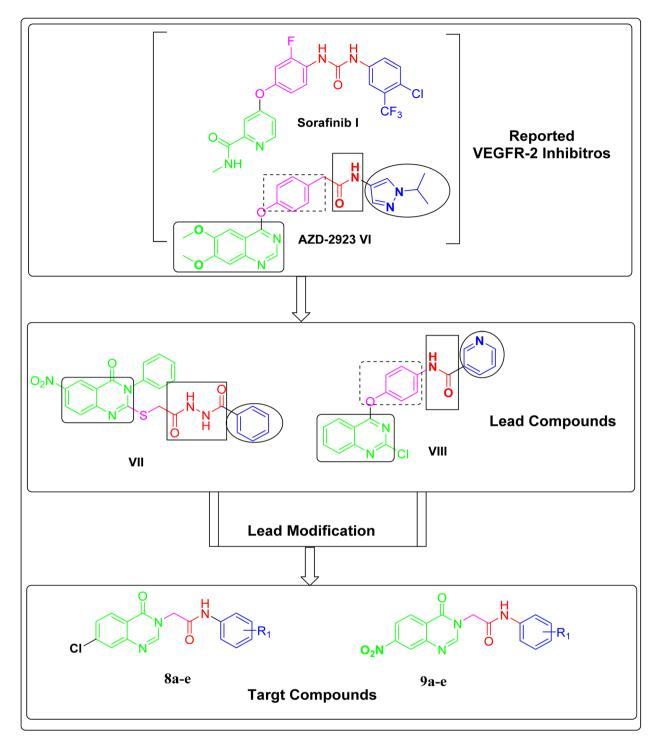
Fig. 2 The proposed design of the target compounds.
