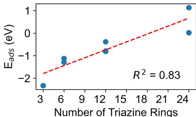
Fig. 8 Correlation between the adsorption energies of  $\text{CO}_2$  over Co/carbon nitrides and the size of the carbon nitride (i.e., number of triazine rings). The red dashed line shows a linear fit.
