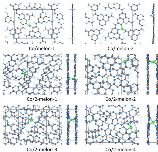
**Fig. 3** Stable structures where Co was bound to melon strands. Brown spheres represent carbon atoms, blue spheres represent nitrogen atoms, pink spheres represent hydrogen atoms, and green spheres represent cobalt atoms. When two melons are present, these are designated by the prefix '2-'. Each unique configuration is identified by the final number (e.g., '-1', '-2', etc.). Top and side views are shown. Simplified images of the Co/melon structures are found in Fig. S4.†
