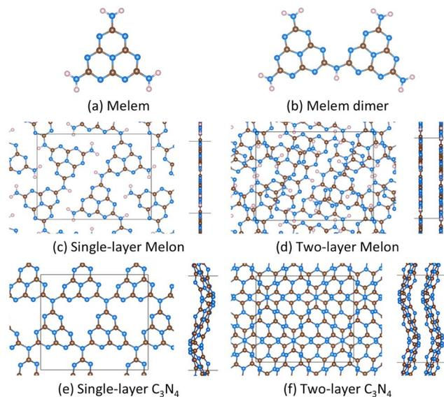
Fig. 1 Carbon nitrides molecules, melem (a) and melem dimer (b), modeled in this work. Periodic carbon nitride polymers, melon (c and d) and graphitic  $C_3N_4$  (e and f), modeled in this work. Also shown are the simulation cells for the periodic structures. Brown spheres represent carbon atoms, blue spheres represent nitrogen atoms, and pink spheres represent hydrogen atoms.
