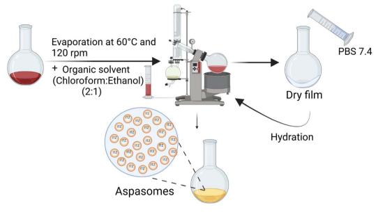
Fig. 5 Method of aspasomal dispersion preparation "thin film hydration method". In the thin film hydration method, the main components of aspasomes (ascorbyl palmitate, phospholipid and cholesterol) are dissolved in a mixture of chloroform: ethanol (2:1). Organic solvent evaporation is performed in a rotary evaporator at 60 °C and 120 rpm. The formed dry thin film is hydrated with phosphate buffer saline (PBS; pH 7.4). This figure was created with BioRender.
