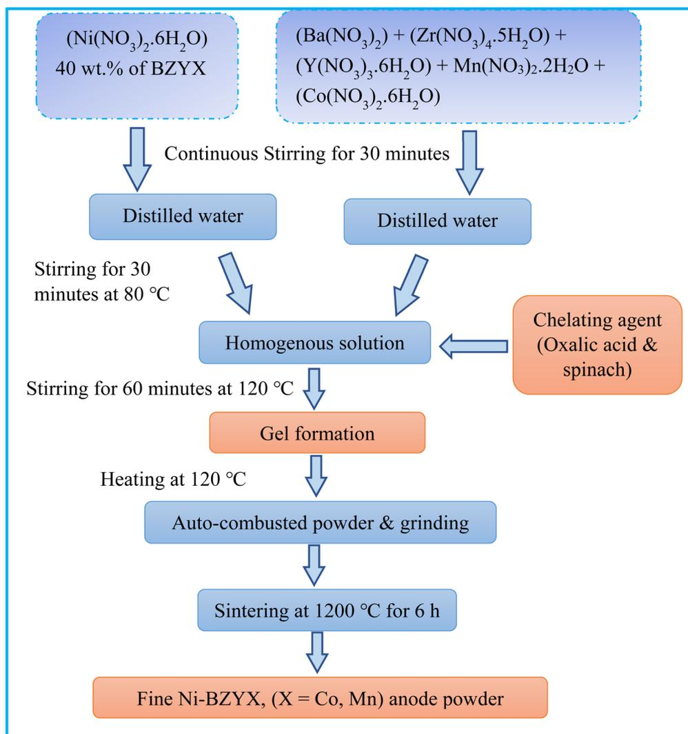
Fig. 1 Flow chart for the Ni-BaZr<sub>0.8</sub>Y<sub>0.1</sub>X<sub>0.1</sub>O<sub>3-δ</sub> (Ni-BZYX, X = Co, Mn) anode synthesis.
