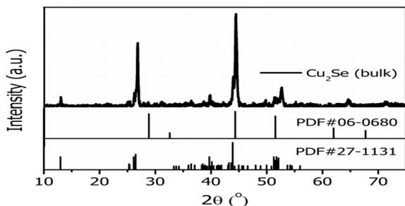
Fig. 2 Room temperature XRD pattern of the bulk  $\text{Cu}_{2-x}\text{Se}$  sample employed for thin film deposition.
