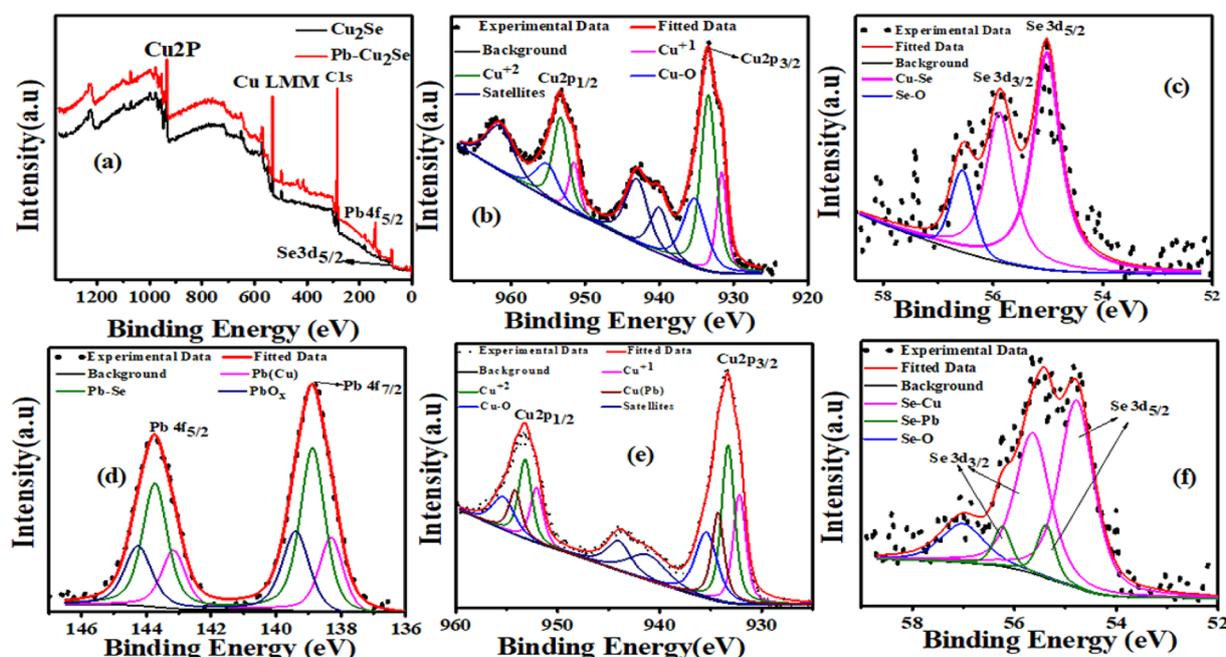
Fig. 3 XPS analysis of  $\text{Cu}_2\text{Se}$  and Pb-5% doped  $\text{Cu}_{2-x}\text{Se}$  thin films. (a) full survey spectra showing elemental peaks. (b, e) Cu 2p spectra, (c, f) Se 3d spectra (d) Pb 4f spectrum for pristine and Pb-doped  $\text{Cu}_{2-x}\text{Se}$  thin films.
