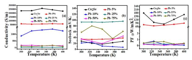
Fig. 6 (a) Shows the temperature-dependent electric conductivity, (b) Seebeck coefficients, and (c) power factor (PF) of all the series of pristine and Pb-doped  $Cu_{(2-x)}$ Se thin films.
