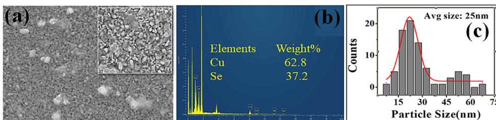
Fig. 4 Surface morphology and compositional analysis of  $\text{Cu}_{2-x}\text{Se}$  thin film. (a) FESEM image showing uniform nanoparticle distribution, with an image in the inset showing clear particle size with a range nearly equal to 100 nm. (b) EDS spectrum confirming the presence of Cu and Se elements in pristine  $\text{Cu}_{2-x}\text{Se}$  thin films. (c) Average particle size  $\sim 25$  nm.
