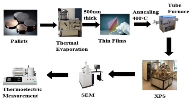
Fig. 1 Schematic diagram of revealing the fabrication and structural and thermoelectric characterization of pristine and Pb-doped Cu<sub>2-x</sub>Se thin films.
