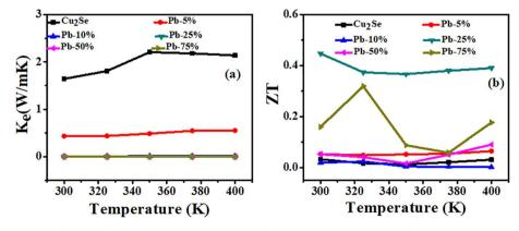
Fig. 7 Temperature-dependent (a) electronic thermal conductivity ( $K_e$ ) and (b) figure of merit (ZT) of all the series of pristine and Pb-doped  $Cu_{(2-x)}$ Se films.
