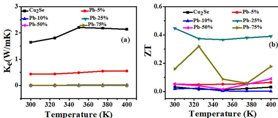
Fig. 7 Temperature-dependent (a) electronic thermal conductivity ( $k_e$ ) and (b) figure of merit (ZT) of all the series of pristine and Pb-doped  $\text{Cu}_{2-x}\text{Se}$  thin films.
