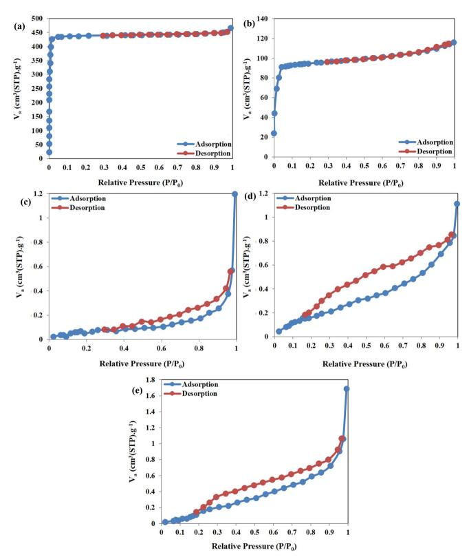
Fig. 3  $N_2$  ad(de)sorption isotherms of (a) ZIF-67, (b) WS/CoFe<sub>2</sub>O<sub>4</sub>/ZIF-67, (c) Hyd, (d) Hyd/WS/CoFe<sub>2</sub>O<sub>4</sub> and (e) Hyd/WS/CoFe<sub>2</sub>O<sub>4</sub>/ZIF-67 nanocomposite samples.
