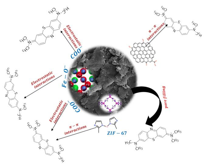
Fig. 11 Scheme of MB adsorption mechanism by Hyd/WS/CoFe<sub>2</sub>O<sub>4</sub>/ZIF-67.
