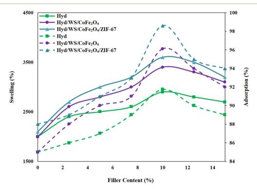
Fig. 5 Impact of filler content on the swelling and removal performance of Hyd/WS, Hyd/WS/CoFe $_2$ O $_4$  and Hyd/WS/CoFe $_2$ O $_4$ /ZIF-67 nanocomposite samples.
