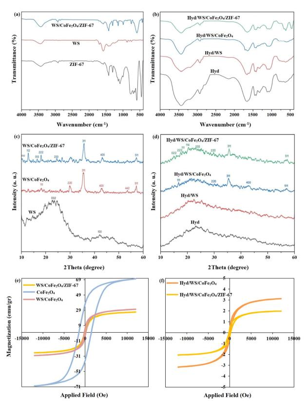
Fig. 2 (a and b) FTIR, (c and d) XRD, and (e and f) VSM analyses of ZIF-67, WS, WS/CoFe<sub>2</sub>O<sub>4</sub>, WS/CoFe<sub>2</sub>O<sub>4</sub>/ZIF-67, Hyd, Hyd/WS, Hyd/WS/ CoFe<sub>2</sub>O<sub>4</sub>, and Hyd/WS/CoFe<sub>2</sub>O<sub>4</sub>/ZIF-67 nanocomposite samples.
