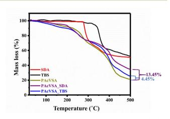
**Fig. 3** Thermogravimetric analysis of SDA, TBS, PAcVSA, PAcVSA\_SDA and PAcVSA\_TBS.
