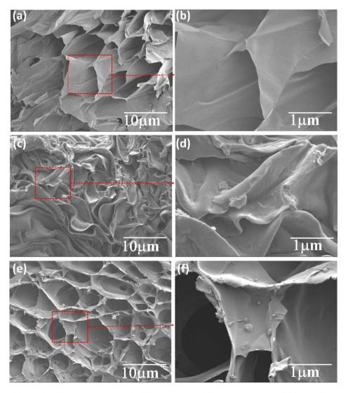
Fig. 4 SEM images of (a) PAcVSA, (b) magnified image of a, (c) PAcVSA\_SDA, (d) magnified image of (c) (red box) showing SDA loading, (e) PAcVSA\_TBS, and (f) magnified image of (e) (red box) showing TBS loading.
