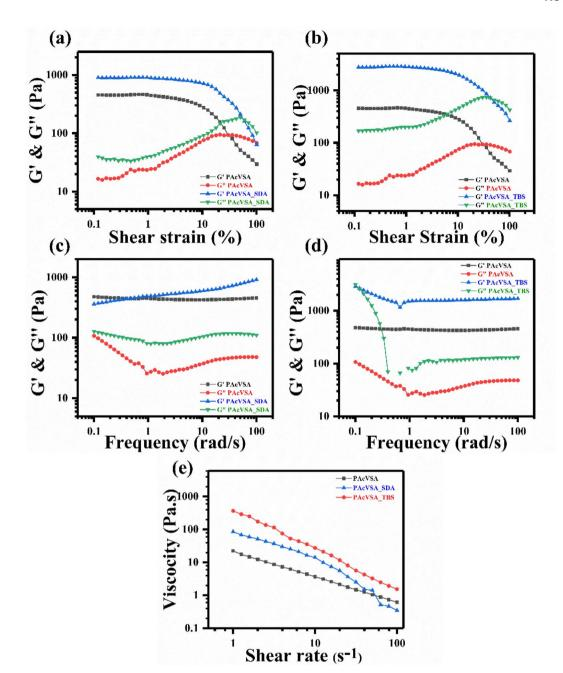
Fig. 5 Rheological properties of PAcVSA, PAcVSA\_SDA and PAcVSA\_TBS hydrogels. (a) and (b) compare the Storage (G') and Loss (G'') modulus of PAcVSA, PAcVSA\_SDA and PAcVSA\_TBS hydrogel with respect to shear strain, respectively, (c) and (d) compare the Storage (G') and loss (G'') modulus of PAcVSA, PAcVSA\_SDA and PAcVSA\_TBS hydrogel with respect to frequency sweep, respectively, (e) shows the shear thinning behaviour of PAcVSA, PAcVSA\_SDA and PAcVSA\_TBS hydrogel.
