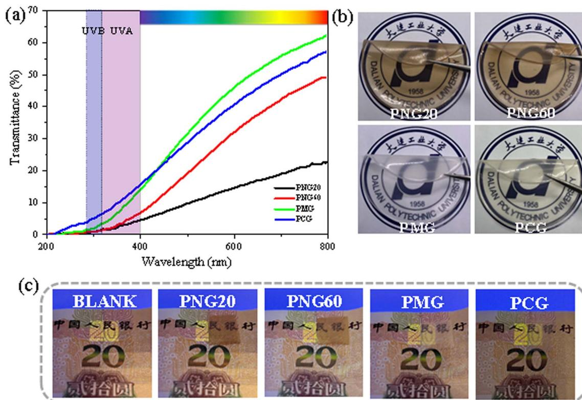
Fig. 5 UV shielding performance (a), optical transparency (b), and UV blocking ability (c) of the prepared composite film.
