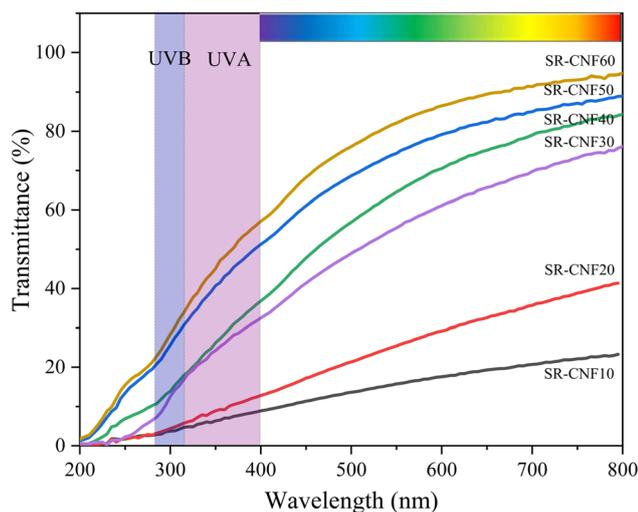
Fig. 4 UV-Visible transmittance of SR-CNF.
