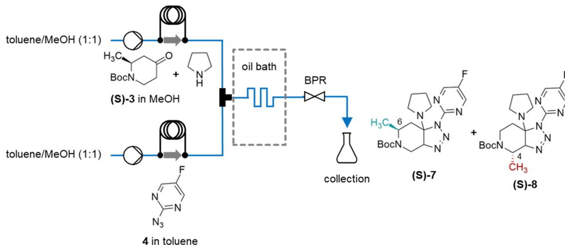
Scheme 2 Continuous-flow experimental set-up for the synthesis of (S)-7 and (S)-8 through cycloaddition (BPR: back pressure regulator).
