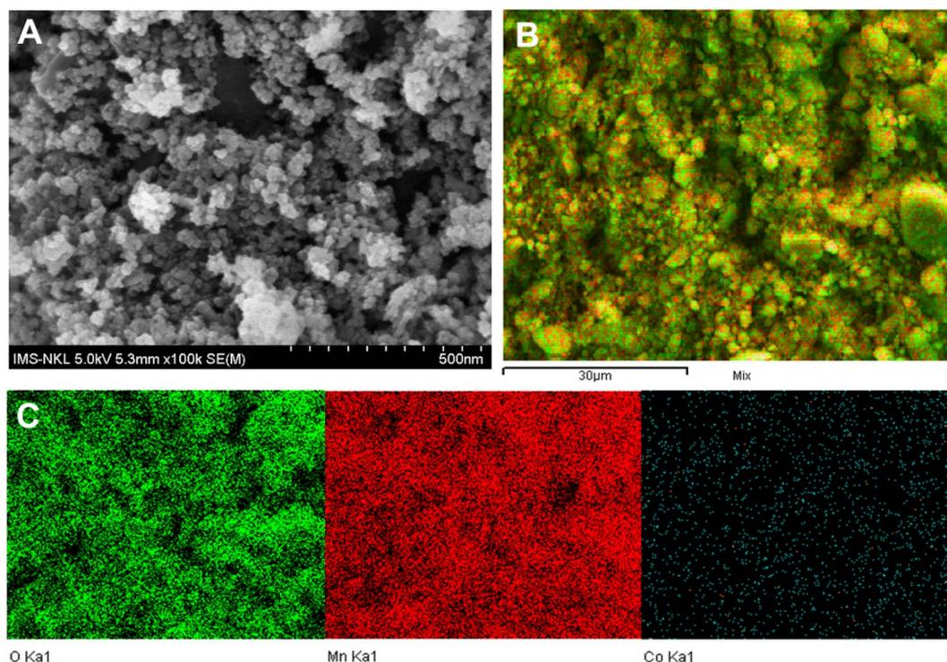
Fig. 1 SEM (A) and EDS Mapping (B and C) of Co–MnO<sub>2</sub> nanoparticles.
