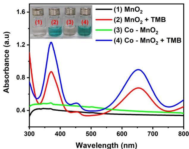
Fig. 3 Absorption spectra and photographs (inset) of (1) MnO<sub>2</sub>, (2) MnO<sub>2</sub> + TMB, (3) Co-MnO<sub>2</sub> and (4) Co-MnO<sub>2</sub> + TMB.
