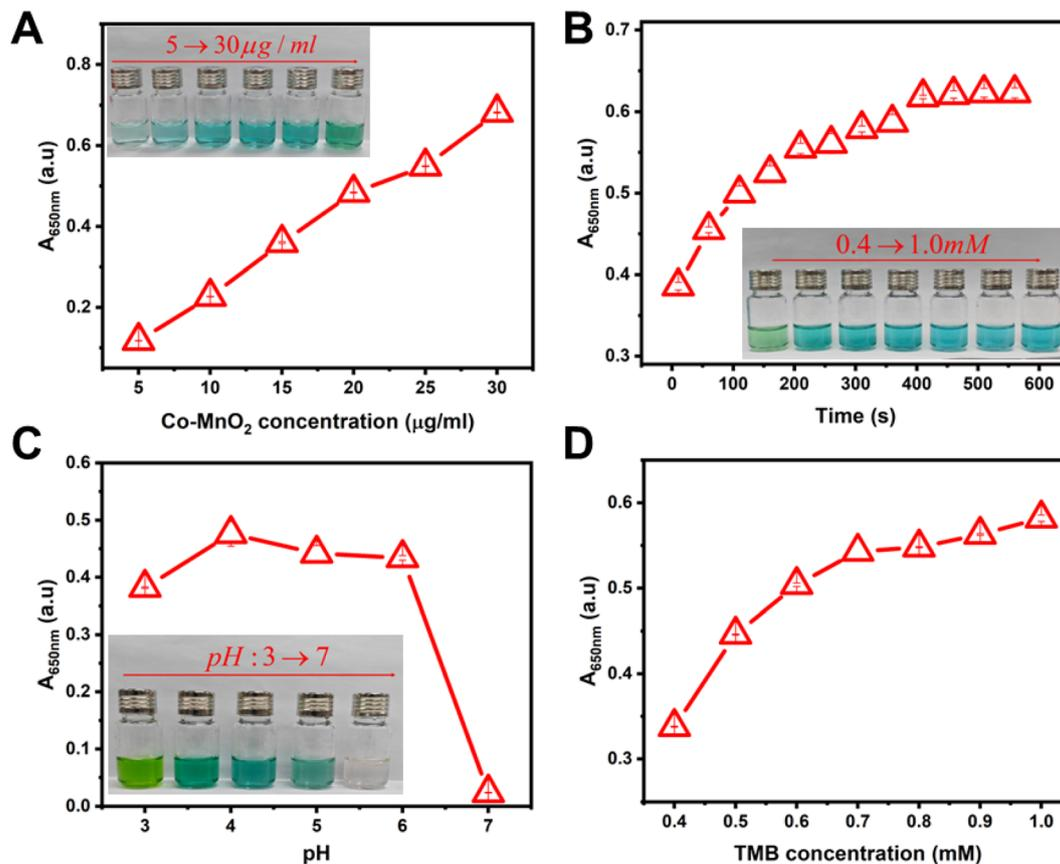
Fig. 4 Oxidase mimetic activity of the Co-MnO<sub>2</sub> is based on (A) concentration of Co-MnO<sub>2</sub>, (B) concentration of TMB, (C) pH, and (D) time. Error bars are for 3 replicates ( $n = 3$ ).
