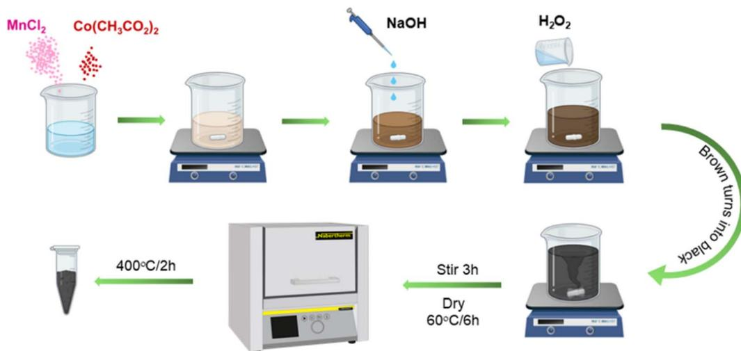
Scheme 1 Process synthesis of Co-MnO<sub>2</sub> nanoparticles.
