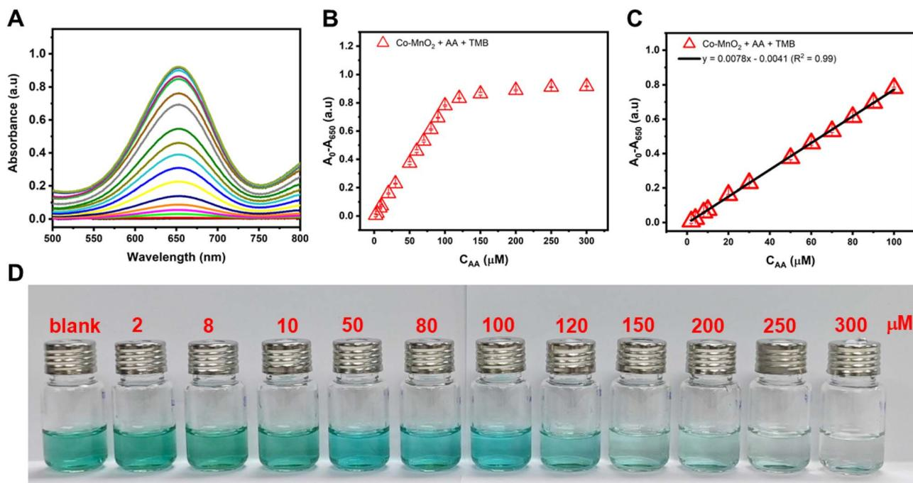
Fig. 6 (A) UV-Vis spectra of Co-MnO<sub>2</sub> + TMB system and (B) plot of dependence of  $\Delta A$  on various concentrations of AA from 0 to 300  $\mu\text{M}$ . (C) Colorimetric detection linear correlation for AA concentrations ranging from 2 to 100  $\mu\text{M}$ . (D) Photo of vials containing Co-MnO<sub>2</sub> + TMB system with different AA concentrations.
