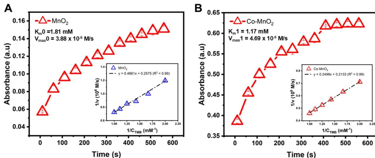
Fig. 5 Plot of absorbance at 650 nm peak versus time of the systems (A) MnO<sub>2</sub> + TMB and (B) Co-MnO<sub>2</sub> + TMB, and Lineweaver-Burk plot (inset), respectively.
