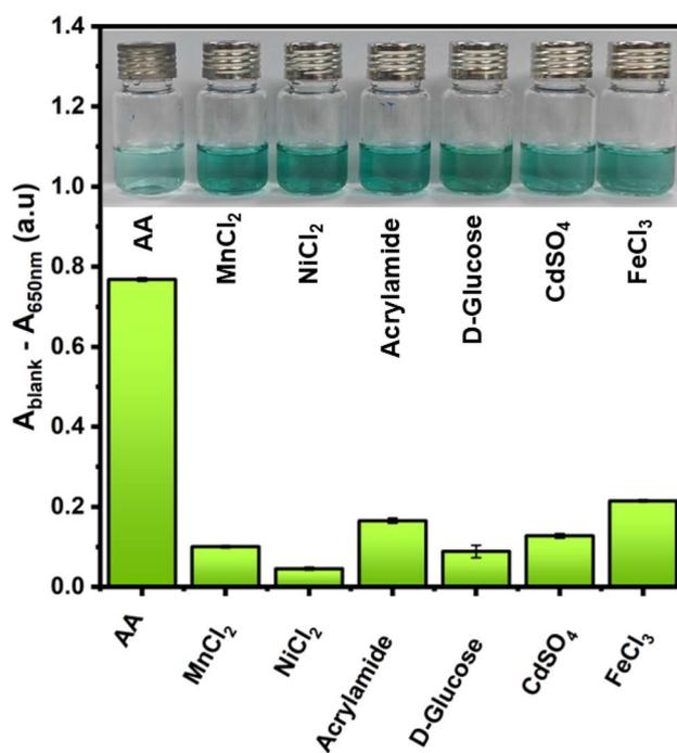
Fig. 7 Selectivity of Co-MnO<sub>2</sub> + TMB system for AA sensing.
