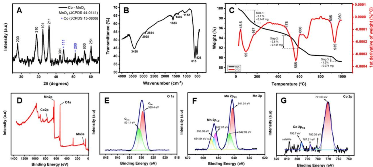
Fig. 2 (A) XRD and (B) FTIR spectrum, (C) TGA and DTG curve of Co-MnO<sub>2</sub> nanoparticles, and (D–G) XPS spectra of Co-MnO<sub>2</sub> nanoparticles.
