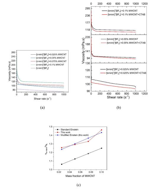
Fig. 6 Viscosity of [bmim]<sup>+</sup>[BF<sub>4</sub>]<sup>-</sup> based Io-Nanofluids (a) effect of MWCNT concentration (b) effect of surfactant CTAB (c) viscosity enhancement with MWCNT concentration.
