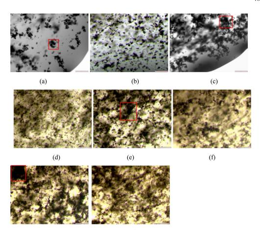
Fig. 9 (a) [bmim][BF<sub>4</sub>] + 0.025% w/w MWCNT (b) [bmim][BF<sub>4</sub>] + 0.025% w/w MWCNT + CTAB (c) [bmim][BF<sub>4</sub>] + 0.05% w/w MWCNT (d) [bmim][BF<sub>4</sub>] + 0.05% w/w MWCNT + CTAB(e) [bmim][BF<sub>4</sub>] + 0.075% w/w MWCNT (f) [bmim][BF<sub>4</sub>] + 0.075% w/w MWCNT (h) [bmim][BF<sub>4</sub>] + 0.1% w/w MWCNT (h) [bmim][BF<sub>4</sub>] + 0.1% w/w MWCNT + CTAB (agglomerations are highlighted in red squares).
