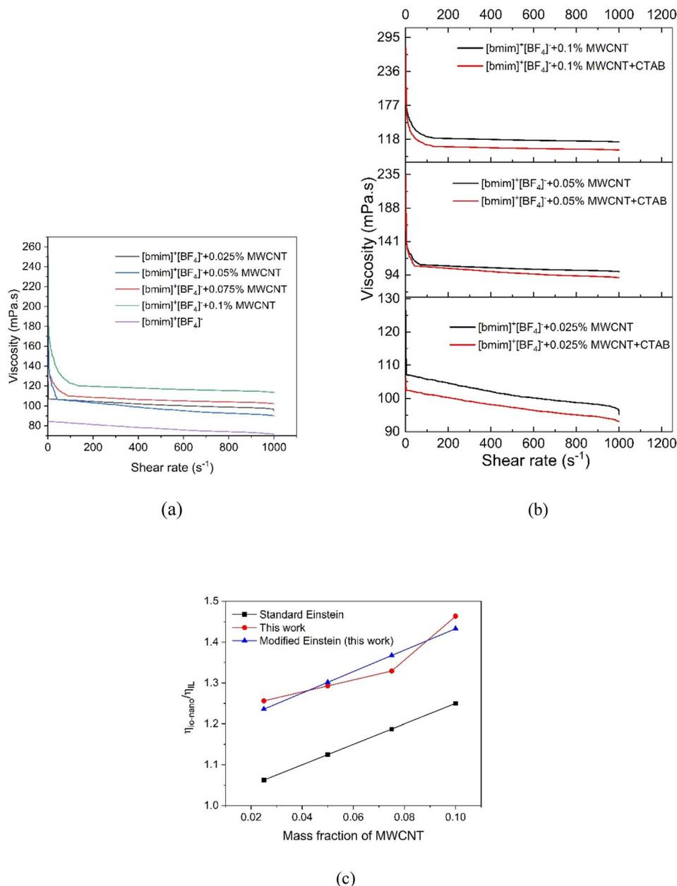
Fig. 6 Viscosity of [bmim]<sup>+</sup>[BF<sub>4</sub>]<sup>-</sup> based Io-Nanofluids (a) effect of MWCNT concentration (b) effect of surfactant CTAB (c) viscosity enhancement with MWCNT concentration.
