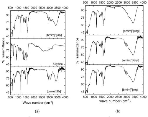
Fig. 2 (a) FTIR of synthesized [bmim]<sup>+</sup>[Gly]<sup>-</sup> with reference to the starting materials [bmim]<sup>+</sup>[Br]<sup>-</sup> and Glycine (b) FTIR of [emim]<sup>+</sup>[Gly]<sup>-</sup>, [emim]<sup>+</sup>[Arg]<sup>-</sup>, [bmim]<sup>+</sup>[Arg]<sup>-</sup>
