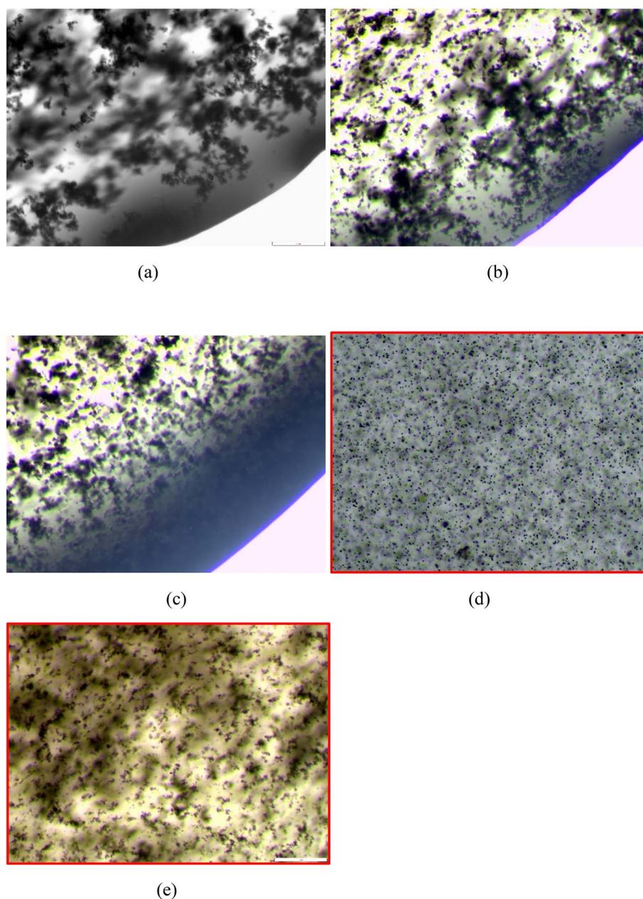
Fig. 5 Effect of surfactant on MWCNT dispersion: (a) [bmim][BF<sub>4</sub>] + 0.05% w/w MWCNT (b) [bmim][BF<sub>4</sub>] + 0.05% w/w MWCNT + Licithin (c) [bmim][BF<sub>4</sub>] + 0.05% w/w MWCNT + SDS (d) [bmim][BF<sub>4</sub>] + 0.05% w/w MWCNT + Tween 80 (e) [bmim][BF<sub>4</sub>] + 0.05% w/w MWCNT + CTAB (better dispersion images highlighted in red).
