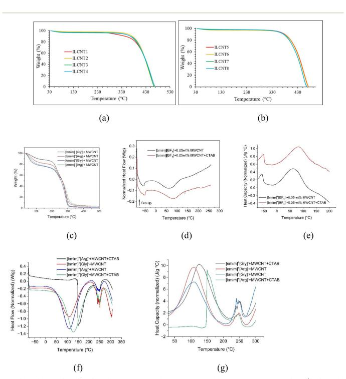
Fig. 8 (a) and (b) TGA of [bmim]<sup>+</sup>[BF<sub>4</sub>]<sup>-</sup> INFs (codes as per Table 2), (c) TGA of AAIL INFs (d) heat flow vs. temperature of [bmim]<sup>+</sup>[BF<sub>4</sub>]<sup>-</sup> INFs (e) heat capacity vs. temperature of [bmim]<sup>+</sup>[BF<sub>4</sub>]<sup>-</sup> INFs (f) heat flow vs. temperature of AAIL INFs (g) heat capacity vs. temperature of AAIL INFs.
