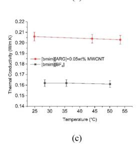
Fig. 13 (a) Comparison of thermal conductivity of Io-Nanofluids (b) enhancement in thermal conductivity of AAIL Io-Nanofluid with respect to [bmim][BF $_4$ ] Io-Nanofluid at 0.05 wt% MWCNT (codes as per Tables 2 and 3) (c) effect of temperature on thermal conductivity.
