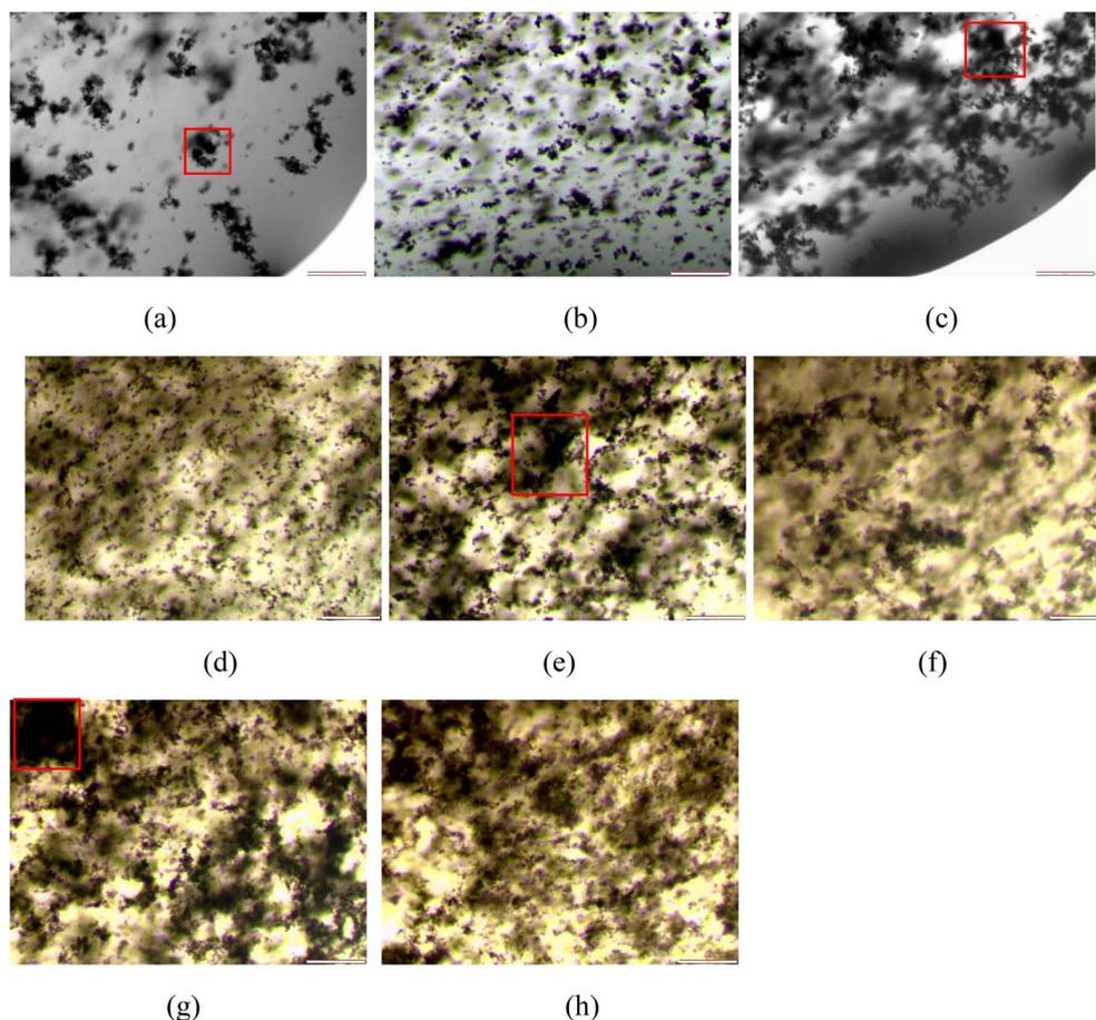
**Fig. 9** (a) [bmim][BF<sub>4</sub>] + 0.025% w/w MWCNT (b) [bmim][BF<sub>4</sub>] + 0.025% w/w MWCNT + CTAB (c) [bmim][BF<sub>4</sub>] + 0.05% w/w MWCNT (d) [bmim][BF<sub>4</sub>] + 0.05% w/w MWCNT + CTAB (e) [bmim][BF<sub>4</sub>] + 0.075% w/w MWCNT (f) [bmim][BF<sub>4</sub>] + 0.075% w/w MWCNT + CTAB (g) [bmim][BF<sub>4</sub>] + 0.1% w/w MWCNT (h) [bmim][BF<sub>4</sub>] + 0.1% w/w MWCNT + CTAB (agglomerations are highlighted in red squares).
