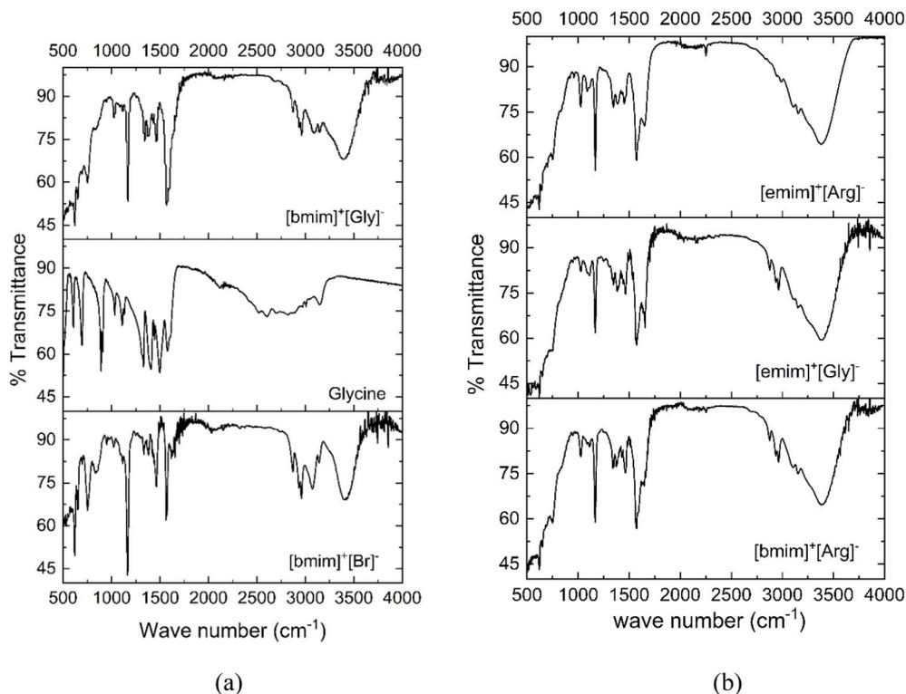
Fig. 2 (a) FTIR of synthesized  $[\text{bmim}]^+[\text{Gly}]^-$  with reference to the starting materials  $[\text{bmim}]^+[\text{Br}]^-$  and Glycine (b) FTIR of  $[\text{emim}]^+[\text{Gly}]^-$ ,  $[\text{emim}]^+[\text{Arg}]^-$ ,  $[\text{bmim}]^+[\text{Arg}]^-$ .
