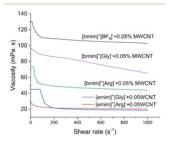
Fig. 7 Shear rate versus viscosity comparision for Io-Nanofluid based on AAIL and [bmim]+[BF<sub>4</sub>]-.
