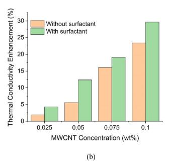
Fig. 11 (a) Thermal conductivity of  $[bmim]^+[BF_4]^-$  based Io-Nanofluid (ILCNT code as per Table 2) (b) thermal conductivity enhancment with respect to pure IL.
