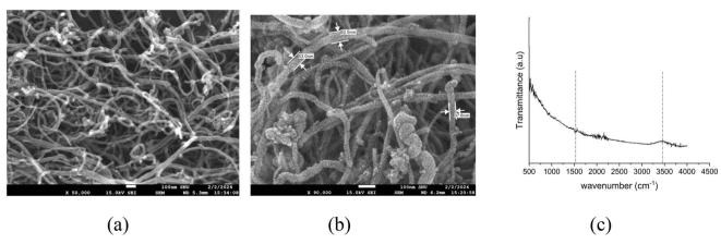
Fig. 1 MWCNT characterization (a) and (b) FESEM (c) FTIR.
