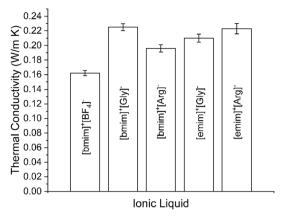
Fig. 12 Thermal conductivity of AAILs in comparision to  $[bmim]^+[BF_4]^-.$
