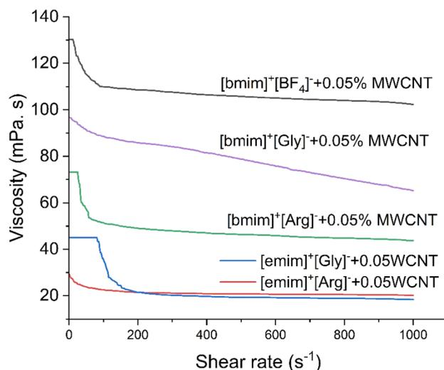
Fig. 7 Shear rate versus viscosity comparison for Io-Nanofluid based on AAIL and  $[\text{bmim}]^+[\text{BF}_4]^-$ .
