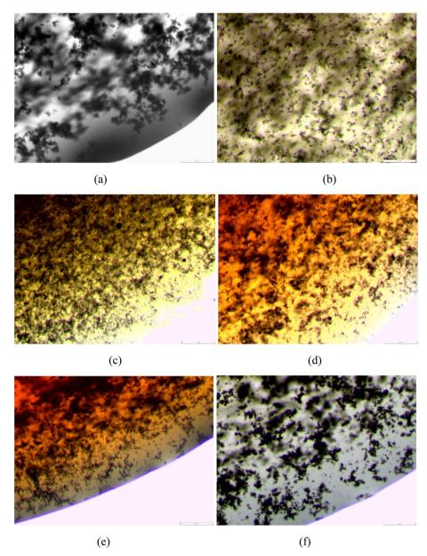
Fig. 10 (a) [bmim][BF<sub>4</sub>] + 0.05% w/w MWCNT (b) [bmim][BF<sub>4</sub>] + 0.05% w/w MWCNT + CTAB (c) [bmim][Arg] + 0.05% w/w MWCNT (d) [bmim][Arg] + 0.05% w/w MWCNT + CTAB (e) [emim][Gly] + 0.05% w/w MWCNT (f) [bmim][Gly] + 0.05% w/w MWCNT + CTAB.
