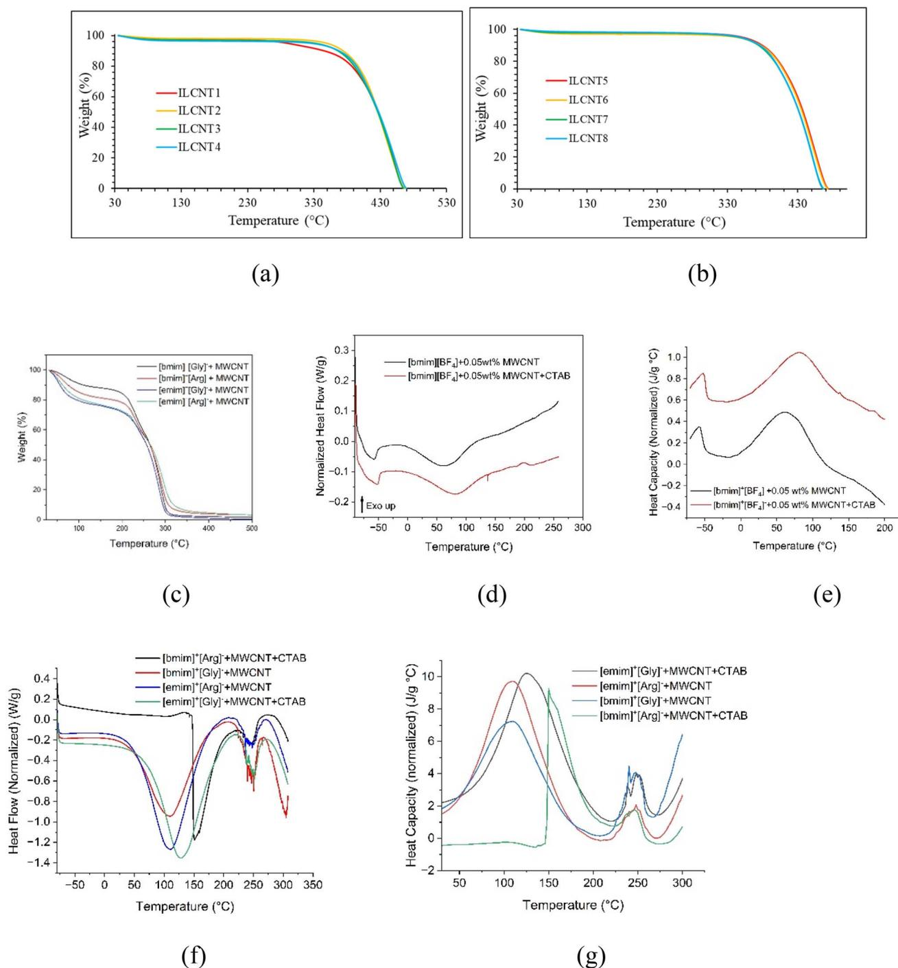
Fig. 8 (a) and (b) TGA of  $[\text{bmim}]^+[\text{BF}_4]^-$  INFs (codes as per Table 2), (c) TGA of AAIL INFs (d) heat flow vs. temperature of  $[\text{bmim}]^+[\text{BF}_4]^-$  INFs (e) heat capacity vs. temperature of  $[\text{bmim}]^+[\text{BF}_4]^-$  INFs (f) heat flow vs. temperature of AAIL INFs (g) heat capacity vs. temperature of AAIL INFs.
