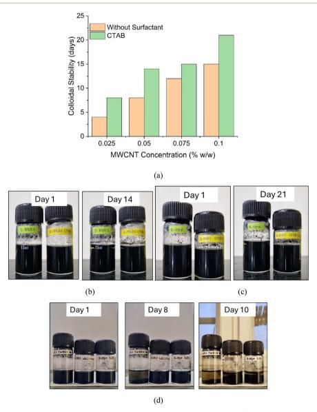
Fig. 14 (a) Effect of MWCNT concentration and CTAB addition on the colloidal stability of [bmim] $^+$ [BF<sub>4</sub>] $^-$  Io-Nanofluids. (b) Colloidal stability of Io-Nanofluid with 0.05 wt% MWCNT (c) colloidal stability of Io-Nanofluid with 0.1 wt% MWCNT (d) colloidal stability of Io-Nanofluid with 0.05 wt% MWCNT with Tween 80. Licithin and SDS.
