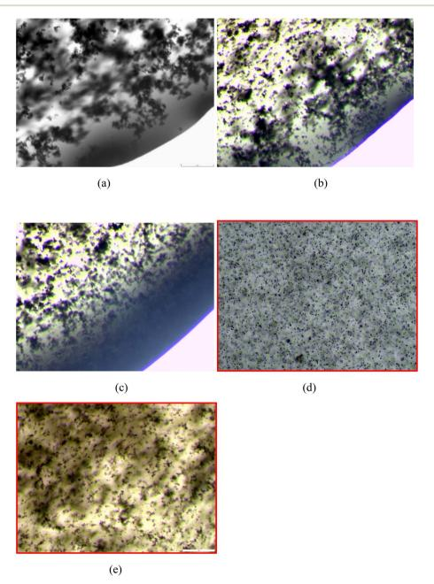
Fig. 5 Effect of surfactant on MWCNT dispersion: (a)  $[bmim][BF_4] + 0.05\%$  w/w MWCNT (b)  $[bmim][BF_4] + 0.05\%$  w/w MWCNT + Licithin (c)  $[bmim][BF_4] + 0.05\%$  w/w MWCNT + SDS (d)  $[bmim][BF_4] + 0.05\%$  w/w MWCNT + Tween 80 (e)  $[bmim][BF_4] + 0.05\%$  w/w MWCNT + CTAB (better dispersion images highlighted in red).
