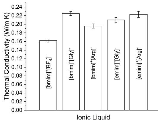
Fig. 12 Thermal conductivity of AAILs in comparison to [bmim]<sup>+</sup>[BF<sub>4</sub>]<sup>-</sup>.
