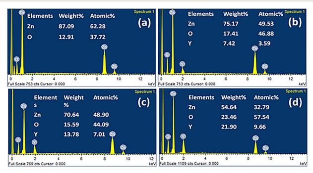
Fig. 6 Energy-dispersive spectroscopy data showing atomic and weight percentages of (a) ZnO and yttrium-doped zinc oxide (b)  $Zn_{0.99}Y_{0.01}O$ , (c)  $Zn_{0.98}Y_{0.02}O$ , (d)  $Zn_{0.97}Y_{0.03}O$ , respectively.
