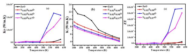
Fig. 9 Electronic thermal conductivity ( $K_e$ ) and total thermal conductivity (K) (a) and (b), estimated (ZT) (c).
