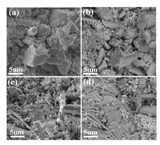
Fig. 4 Secondary electron (a) and BSE (b) images of the Zn<sub>0.99</sub>Y<sub>0.01</sub>O (Y-1%), and the corresponding images for the  $Zn_{0.97}Y_{0.03}O$  (Y-3%) sample are given in (c) and (d), respectively.
