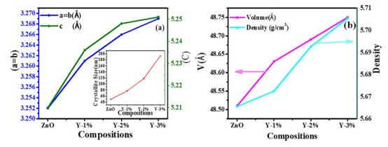
Fig. 3 (a) Lattice parameters a = b and c of ZnO and Y-doped ZnO as a function of yttrium (Y) concentration, showing a gradual increase with doping, where, crystallite size vs. doping concentration is given in the inset. (b) Unit cell volume and theoretical density of ZnO and Y-doped ZnO, both showing a rising trend with increasing Y content.
