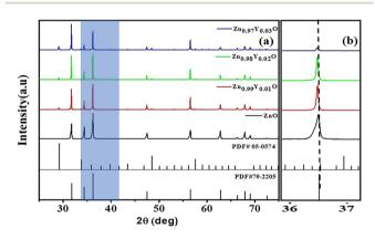
Fig. 2 (a) XRD spectra of ZnO,  $Zn_{0.99}Y_{0.01}O$ ,  $Zn_{0.98}Y_{0.02}O$ , and Zn<sub>0.97</sub>Y<sub>0.03</sub>O showing phase evolution and crystallinity. Standard JCPDS patterns for ZnO (01-079-2205) and  $Y_2O_3$  (05-0574) are included for reference. (b) Magnified image of peaks shifting.
