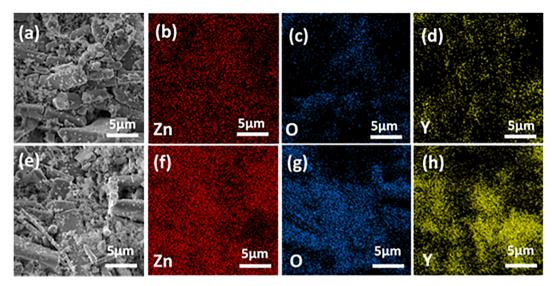
Fig. 5 Backscattered electron (BSE) image (a) along with EDS elemental mapping (b-d) of  $Zn_{0.98}Y_{0.02}O$ , and BSE image (e) along with EDS elemental mapping (f-h) of  $Zn_{0.97}Y_{0.03}O$ .
