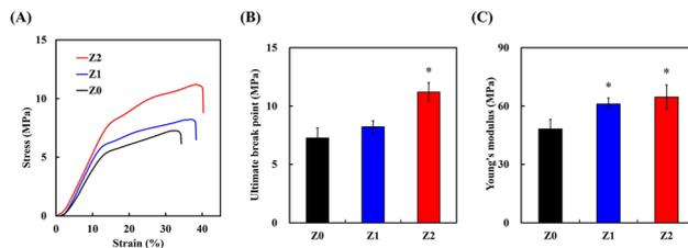
Fig. 5 (A) Compressive stress–strain curves of as-printed scaffolds. (B) Comparison of ultimate compressive strength. (C) Comparison of Young's modulus across different scaffold formulations. \* indicates statistically significant differences compared to Z0 ( $p < 0.05$ ). Data represent the mean  $\pm$  SD of 6 measurements.
