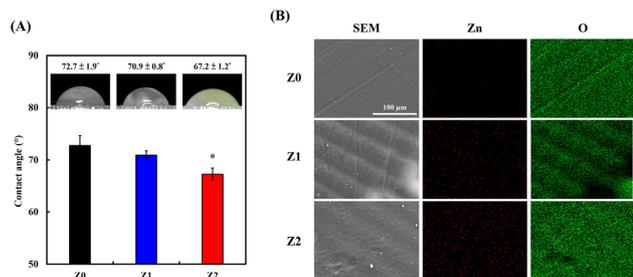
Fig. 4 (A) Contact angle measurements of PU scaffold surfaces with inset droplet profiles. (B) SEM micrographs and EDX elemental maps of Zn and O for Z0, Z1, and Z2 surfaces. \* indicates statistically significant differences compared to Z0 ( $p < 0.05$ ). Data represent the mean  $\pm$  SD of 6 measurements.
