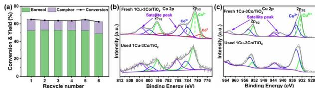
Fig. 4 The recyclability of the 1Cu-3Co/TiO<sub>2</sub> catalyst. (a) Catalytic performance, (b) Co 2p and (c) Cu 2p XPS spectra of 1Cu-3Co/TiO<sub>2</sub> before and after reaction. Reaction conditions: 0.25 g catalyst, 3 MPa H<sub>2</sub>, 160 °C, 30 mL heptane, 0.5 g isoborneol, 2 h.
