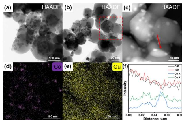
**Fig. 3** TEM characterizations of 3Co/TiO<sub>2</sub> and 1Cu–3Co/TiO<sub>2</sub>. (a) HAADF-STEM image of Co/TiO<sub>2</sub>. (b and c) HAADF-STEM image of 1Cu–3Co/TiO<sub>2</sub>. (d and e) EDS mapping patterns of Co and Cu over 1Cu–3Co/TiO<sub>2</sub>. (f) Line-scanning elemental distribution for 1Cu–3Co/TiO<sub>2</sub> along the red arrow in (c).
