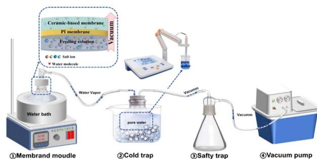
Fig. 1 Schematic diagram of the PV separation apparatus.
